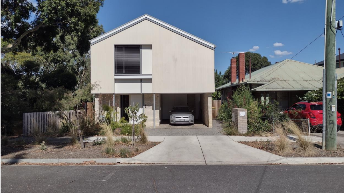
Western Façade of the dwelling, showing integration of carport to form of dwelling
