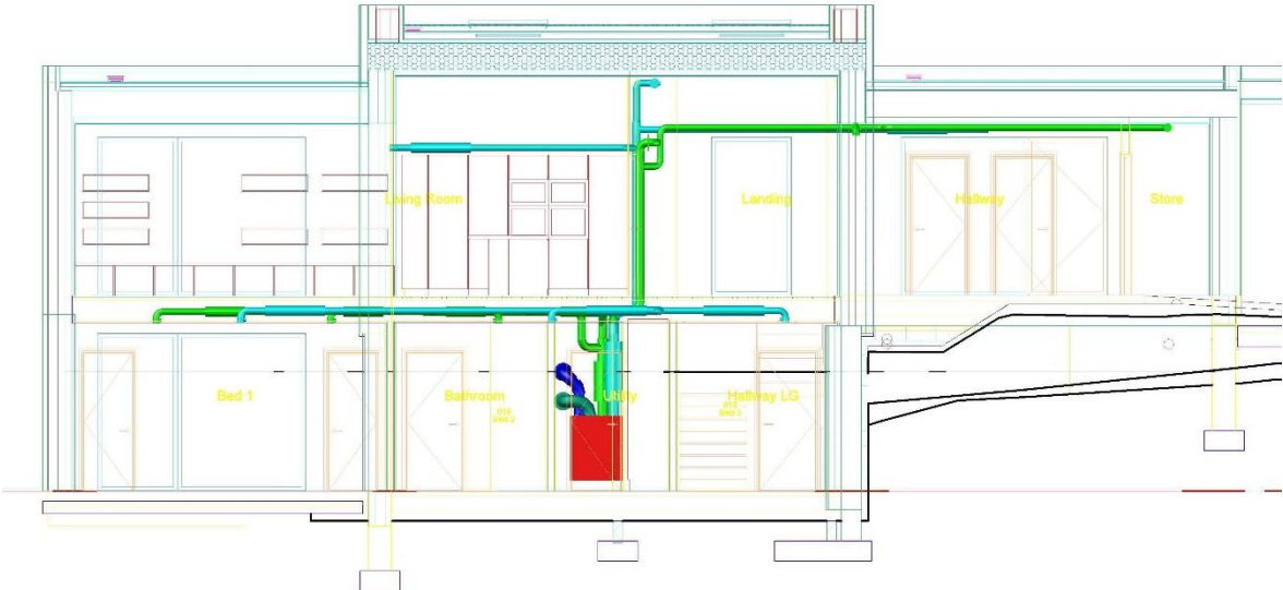
Section showing MVHR layout (by GBS based on our initial MVHR layout)
