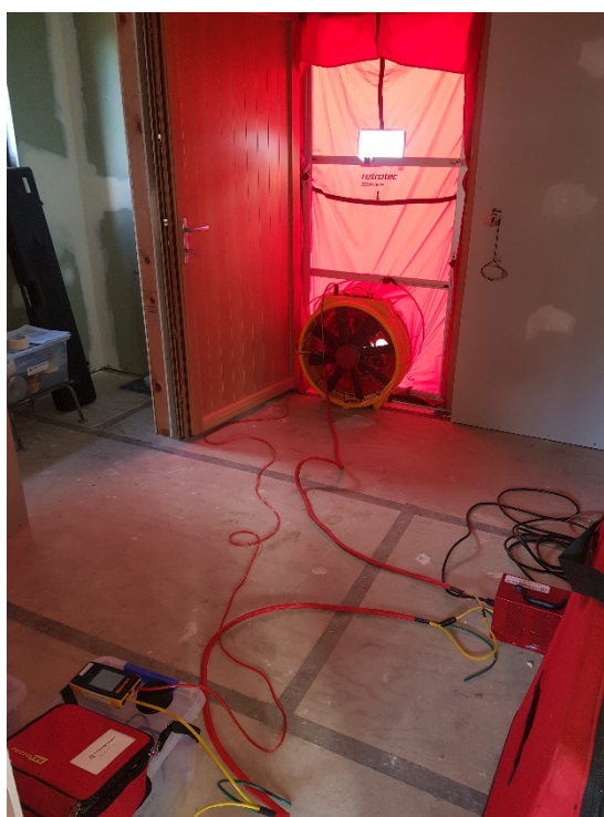
Figure 23 Blower Door Test in progress
