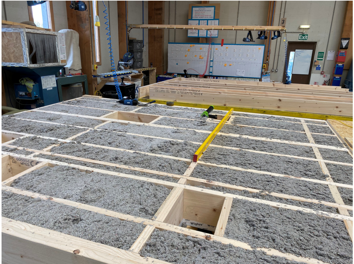
Wall panel during factory construction with all cavities filled with Warmcel cellulose insulation (Panel uncovered for photograph, typically Warmcel pumped to a density of 65kg/m 3 to meet requirements for off-site transportation).
