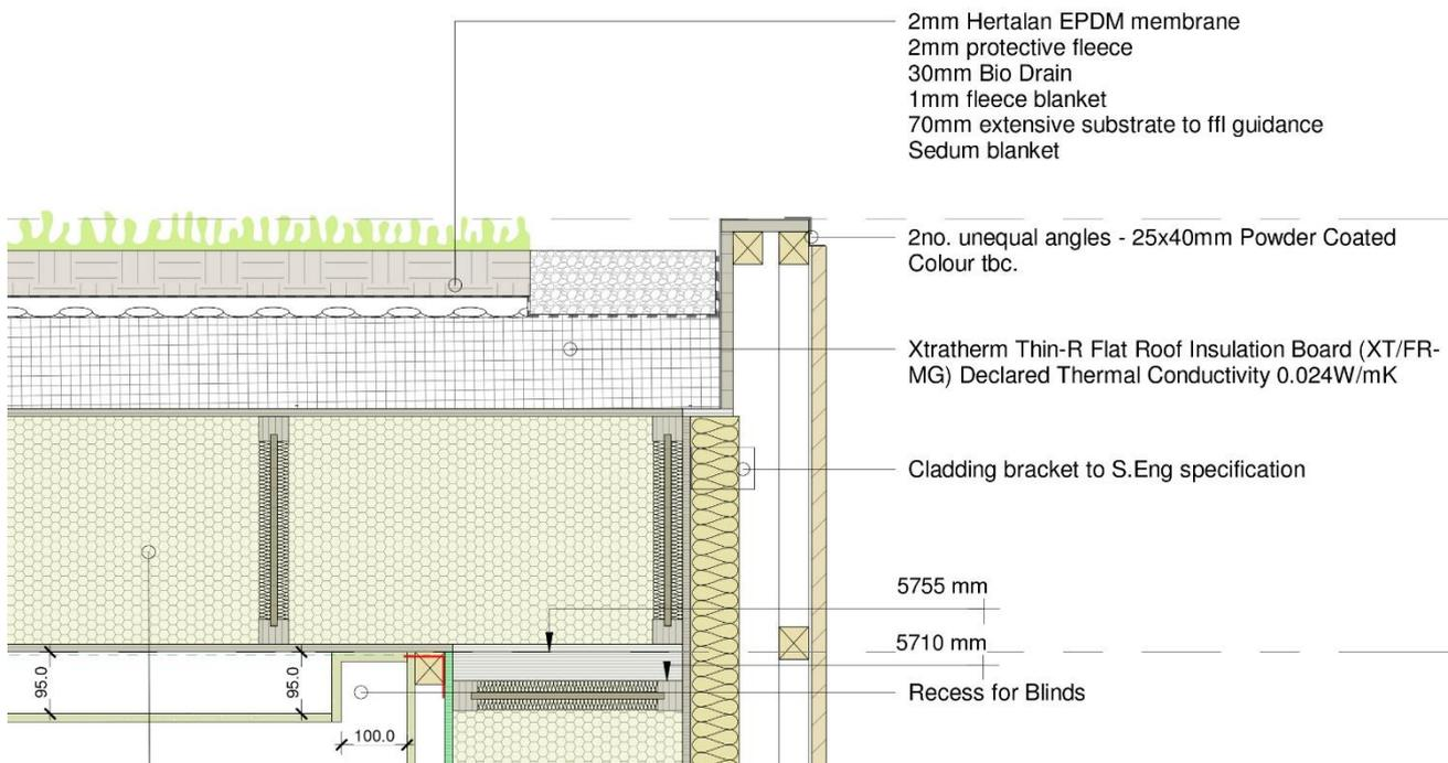
The Roof has full fill timber frame with rigid insulation on top, to provide a super insulated roof structure. There is then a green roof over the EPDM membrane.
