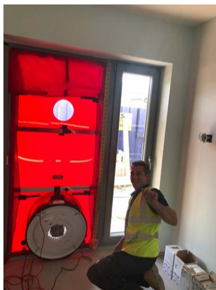
Photograph of airtightness testing, with Jason Harrison/Tuakana, Airtightness Champion on site
