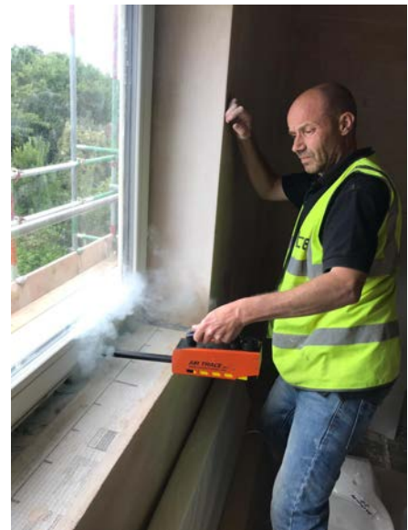
Photograph of airtightness (smoke gun) test of window installation by Simon Freeley, BRE
