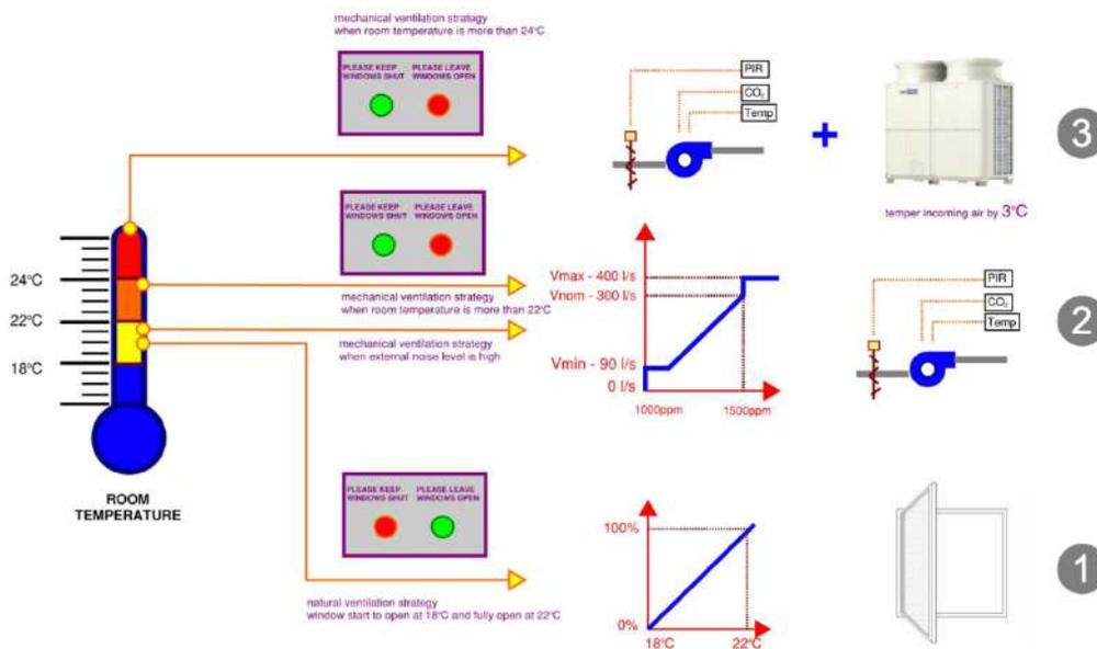
Each classroom has a “Window Open/Close” indicator installed next to the teacher’s desk – visible to teachers and pupils. The unit indicates that windows can be opened when outdoor temperatures are appropriate if interior temperatures exceed 18°C or CO<sub>2</sub> levels are high to optimise thermal comfort whilst minimising risk of energy loss through windows.
