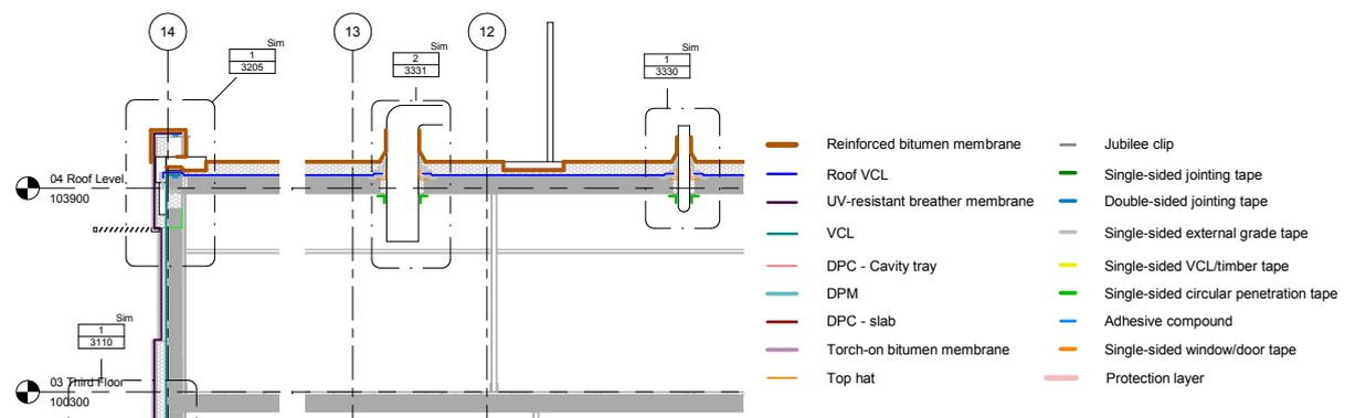
Detailed section showing the membranes and airtightness products used to ensure roof penetrations were made airtight.
