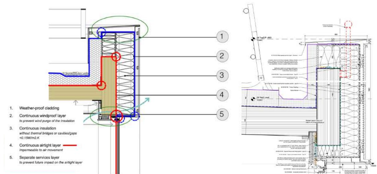
Detailed section from early planning stage (left) and construction stage (right) highlighting critical components of the parapet detail to ensure it's built to be airtight and thermally continuous.
