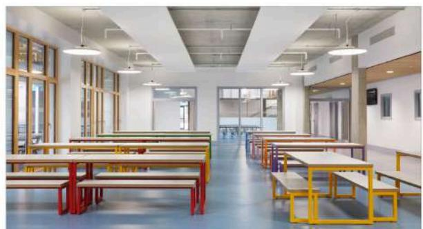
Bottom right: Dining space with exposed concrete soffit on ground floor to benefit from thermal mass.
