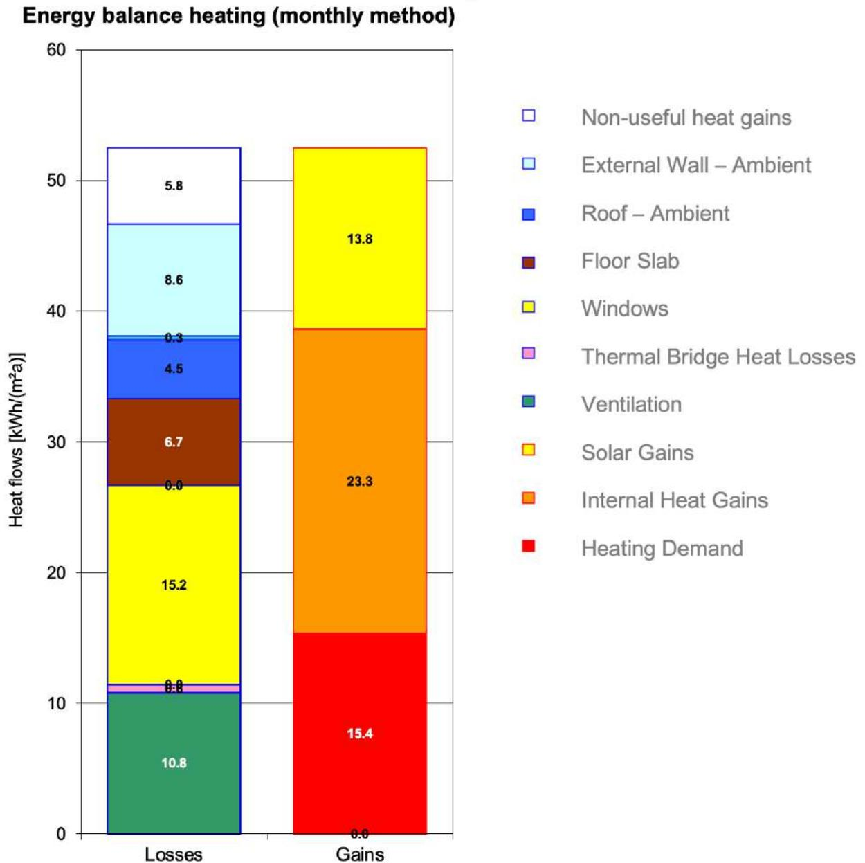
The Energy Balance graph shows the breakdown of losses and gains. The windows account for roughly a third (29%) of the heat losses across the building however they also contribute roughly a third (26%) in solar gains. This balance was carefully managed through optimising the glazing and shading design to provide useful solar gains in winter, and minimising risk of overheating in warmer months.
