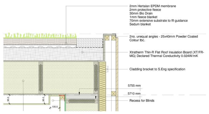
The Roof has full fill timber frame with rigid insulation on top, to provide a super insulated roof structure. There is then a green roof over the EPDM membrane.
