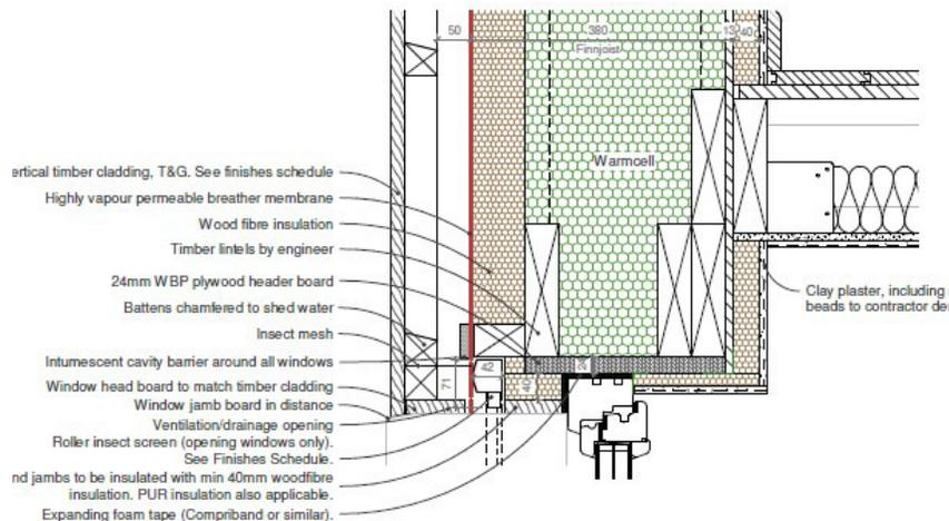
Both the wall and the roof are constructed from 300mm deep timber I-joists filled with Warmcel insulation (blown cellulose) with 80mm wood fibre insulation (Steico Special Dry) and timber cladding on battens applied externally. Internally, 12mm Pro-Passive OSB, with 40mm wood fibre (Steico Internal) with clay plaster.
