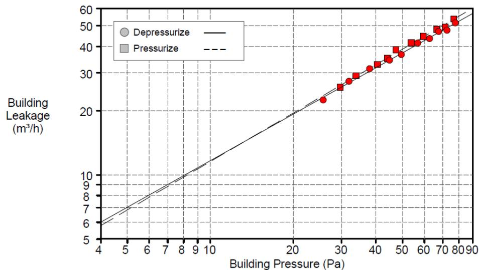
The air pressure test was carried out by Elmhurst Energy on 1st August 2022. A previous air-pressure test was carried out 3 months before once the airtightness layer was complete, and before installing internal linings such as the clay plaster etc.. The test concluded an Average Air Changes per Hour (n<sub>50</sub>) of 0.135h<sup>-1</sup> @ 50Pa.
