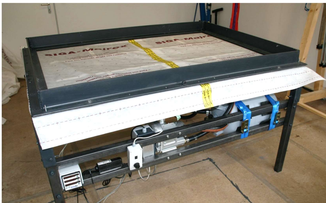
Fig. 5: Test apparatus with clamped membrane (membrane to membrane bonding using Sicrall)
