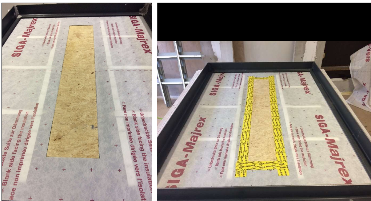
Fig. 2: Cut out membrane with OSB panel (left). OSB panel joined to the membrane on all four sides using Sicrall® (right).
