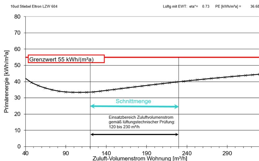
Figure 2: Application range of the unit Stiebel Eltron LZW 604
