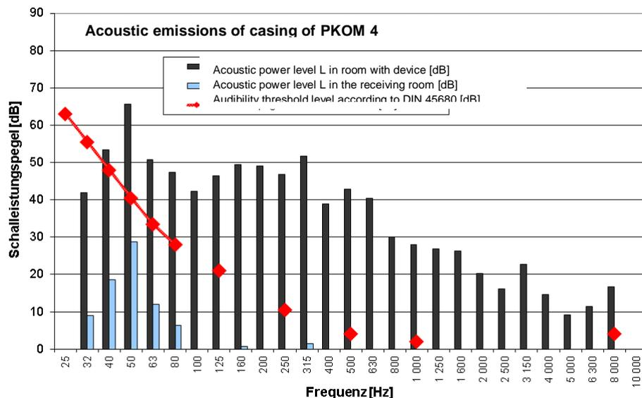
Figure 1: Noise emission of casing of unit PKOM4
