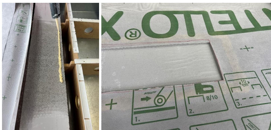
Fig. 3: Membrane to concrete connection using ORCON CLASSIC in the test apparatus (left). Membrane to concrete connection in detail (right).
