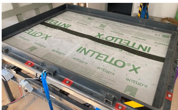
Fig. 1: Connection membrane to membrane with CONTEGA SOLIDO IQ in the test apparatus.
