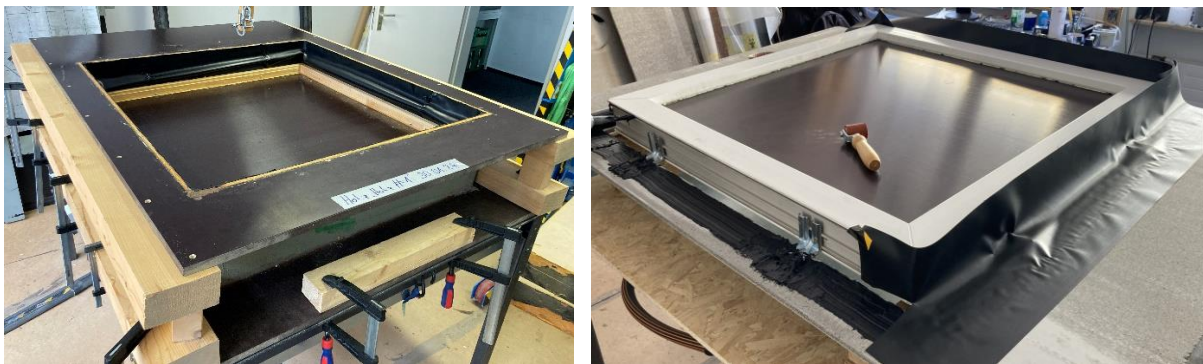
Fig. 1: Wall systems in timber (left) and solid construction (right) with mounting brackets for installing the window frames. The installation areas for the window frames each have a clear dimension of 1030 x 1030 mm.
