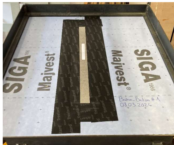
Fig. 1: Setup in the test apparatus with the concrete slab in position. The fixture for the panels simultaneously serves to support the membrane at negative pressure. Bonding of the concrete with the membrane using Trestard 150.
