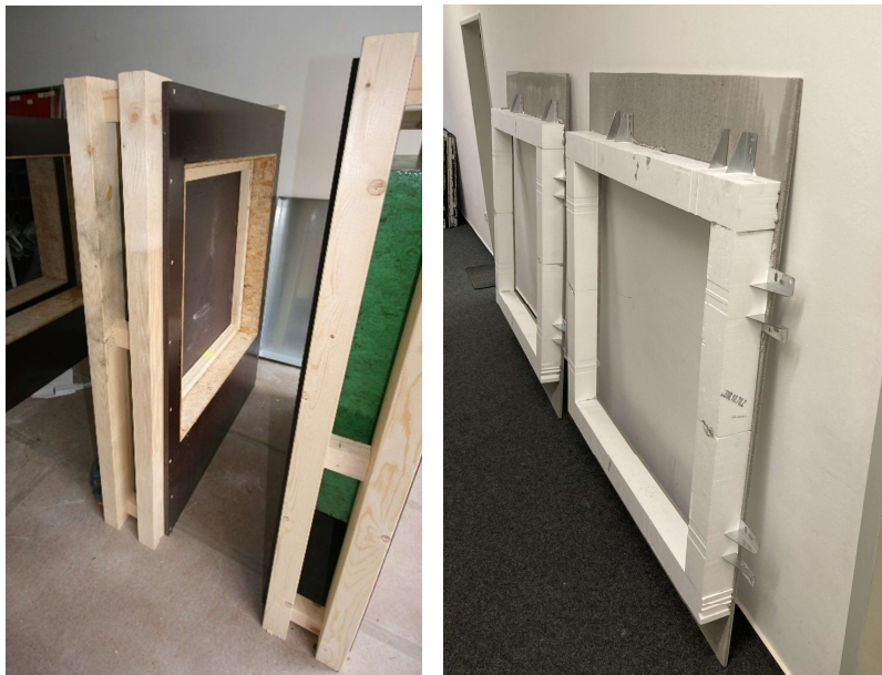
Fig. 1: Wall systems in timber (left) and solid construction (right) with pre-wall installation system for installing the window frames. The installation areas for the window frames each have a clear dimension of 1030 x 1030 mm.
