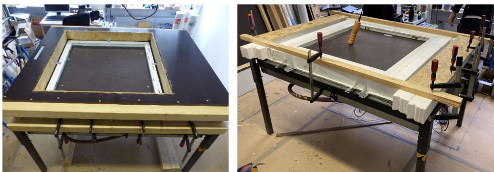
Fig. 3: Measuring device with a laminar flow element with wooden wall section (left) and solid wall section (right)
