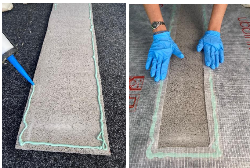
Fig. 3: Membrane to concrete connection using Colle d'étanchéité pare-vapeur Ubbink in the test apparatus (left). Membrane to concrete connection in detail (right).
