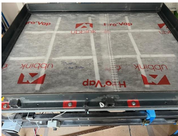
Fig. 1: Connection membrane to membrane with Adhésif Ubbink intérieur in the test apparatus.
