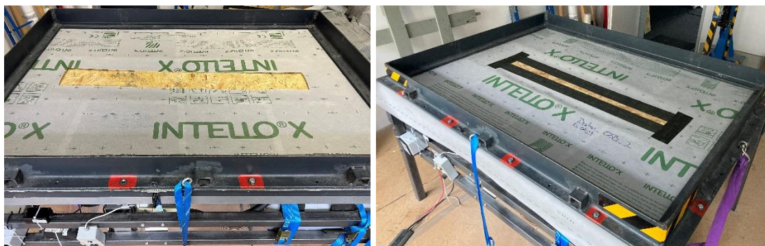
Fig. 2: Cut out membrane with OSB panel (left). OSB panel joined to the membrane on all four sides using Adhésif Ubbink extérieur (right).
