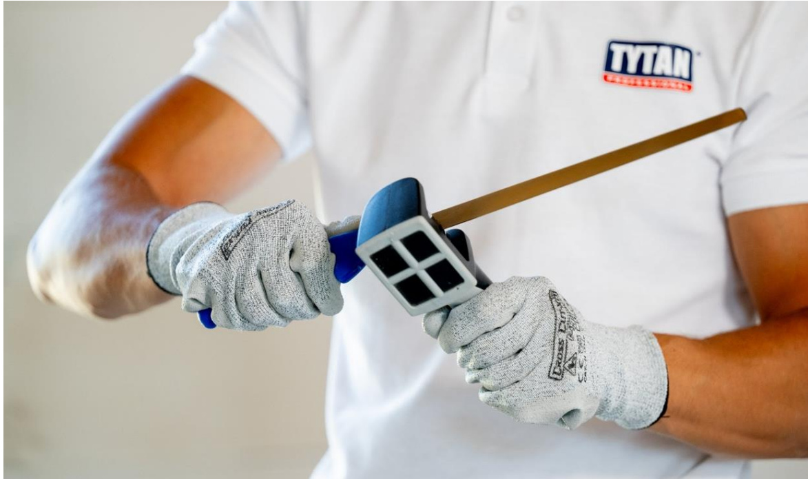
Picture no 10. Before using the TYTAN knife for the first time, prepare the blade to the appropriate sharpness using a sharpener
