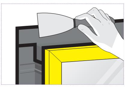
Tool off the paste adhesive with a OBEX CORTEX  $^{\odot}$  0809 Paste Adhesive Spreader to ensure there are no open edges.
