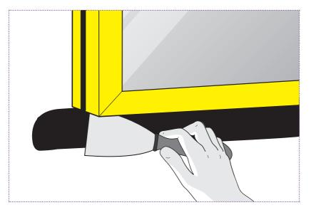
Spread out the paste adhesive evenly using a OBEX CORTEX  $^{\odot}$  0809 Paste Adhesive Spreader making sure you can achieve the correct bond width.
