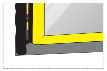
Spread out the paste adhesive evenly using a OBEX CORTEX  $^{\otimes}$  0809 Paste Adhesive Spreader making sure you can achieve the correct bond width.
