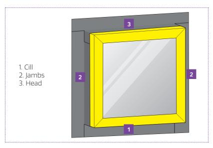
OBEX CORTEX  $^{\odot}$  0500FR Class B Interface Sealing Membrane should be fitted in this order around the window; cill, jambs and then the head.
