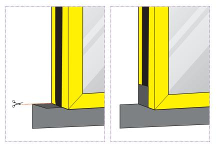
Create an incision along the red dotted line. Now bond the OBEX CORTEX $^{\otimes}$  0500FR Class B Interface Sealing Membrane flap to the sides of the frame, ensuring the membrane is applied flat and without creases.
