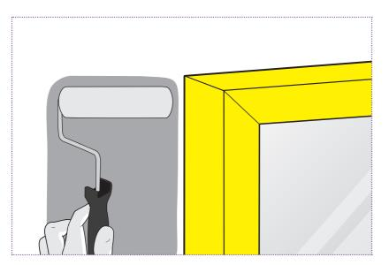
Ensure all substrates are clean, dry and free from grease and oil prior to application. All porous surfaces should be primed using OBEX CORTEX $^{\odot}$  0787FR Non-Flammable Surface Primer.
