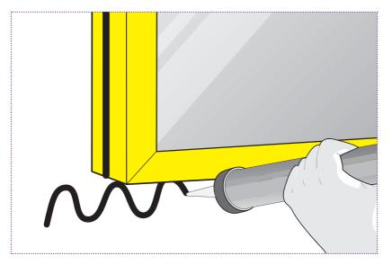
Apply OBEX CORTEX® 0771FR Class B Paste Adhesive to both the frame and the substrate using the OBEX CORTEX® 0813 Paste Adhesive Gun.
