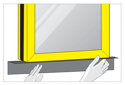
Bond the OBEX CORTEX<sup>®</sup> 0500FR Class B Interface Sealing Membrane to the frame first and then bond back to the substrate, ensuring the membrane is applied flat and without creases. It is important to ensure the cill membrane is fitted first.
