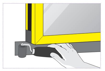
Roll firmly with a OBEX CORTEX 0803 seam roller to ensure maximum bond strength on both the frame and the substrate.
