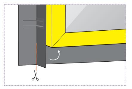
Now apply your second piece of membrane following steps 3-5. Once applied, cut along the red dotted line and fold the flap up to meet the frame. Roll membrane firmly with a OBEX CORTEX 0803 seam roller to ensure maximum bond strength.
