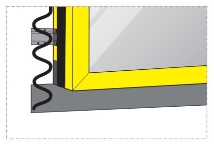
Apply OBEX CORTEX® 0771FR Class B Paste Adhesive to the substrates either side of the window using the OBEX CORTEX® 0813 Paste Adhesive Gun.
