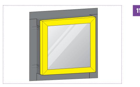
Once all the membrane is bonded, the fold and lap created corners should appear like the above. Apply a further bead of OBEX CORTEX $^{\odot}$  0771FR Class B Paste Adhesive around the perimeter of the membrane and any joints/laps.
