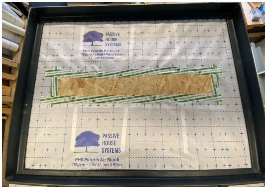
Fig. 3: OSB panel joined to the membrane on all four sides using PHS Argo Plus (Joint Tape).
