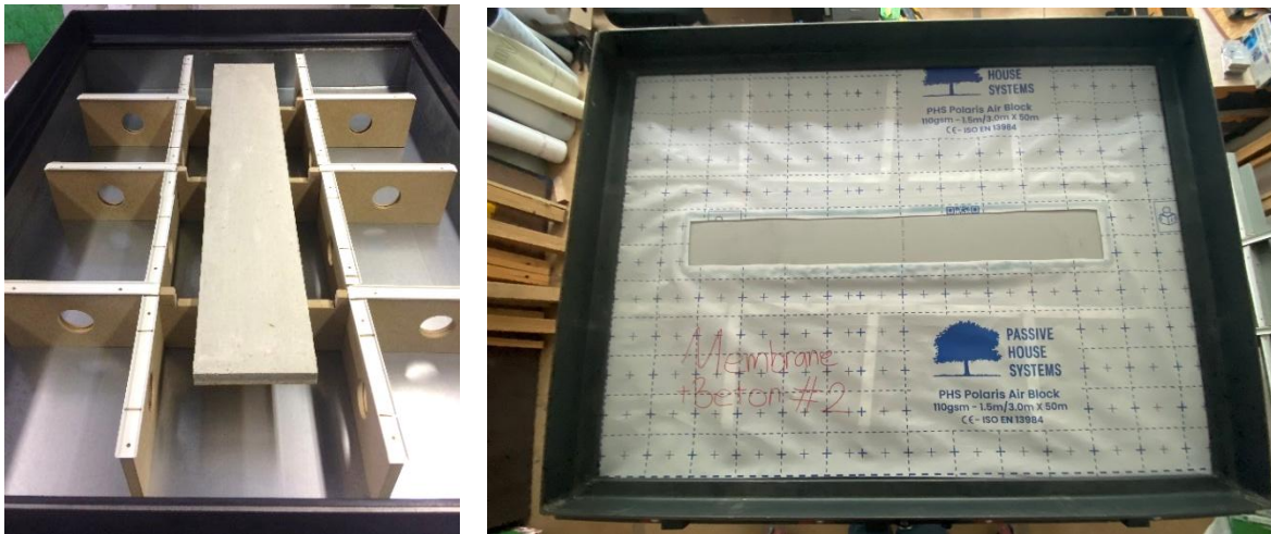
Fig. 2: Fixture for panels in the test apparatus with the concrete slab in position (left). The fixture for the panels simultaneously serves to support the membrane at negative pressure. Adhesion of the concrete with the membrane using PHS Ottello (Adhesive Sealant) (right).
