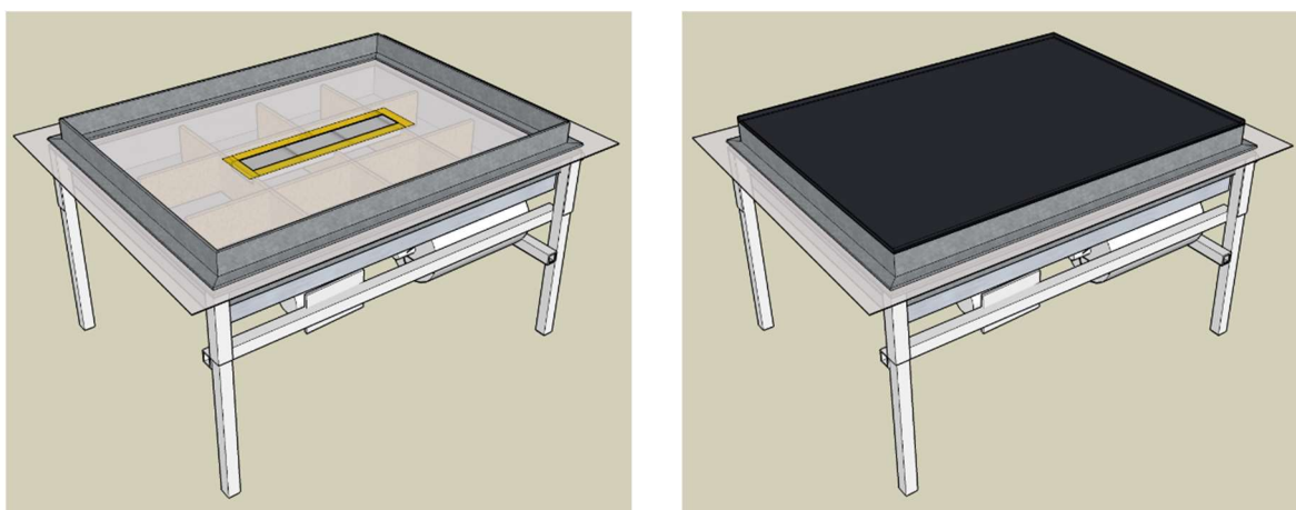
Fig 7: Sketch of the test apparatus with the clamped membrane and inserted panel which is joined to the membrane with adhesive tape (yellow) (left). Test apparatus sealed with the cover panel for determining the test stand leakage (right).
