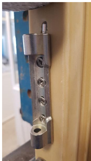
Shear test with tearing and breakage of the guide pin
