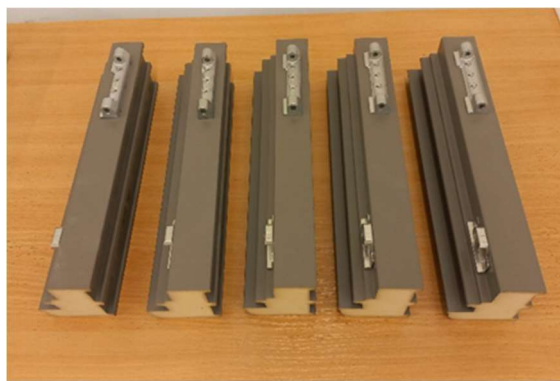
Figure 1 IWF-16: samples of window frame for the tests
