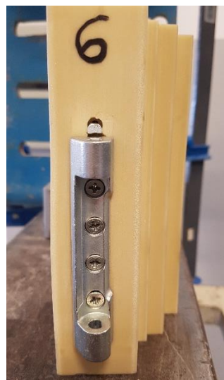
Shear test with tearing and breakage of the guide pin
