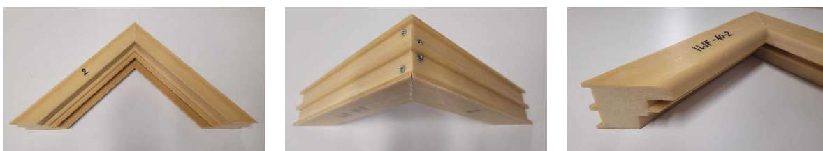
Figure 2 IWF-10: samples of window frame for the tests
