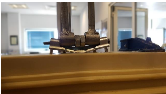
Pull-off tensile test
