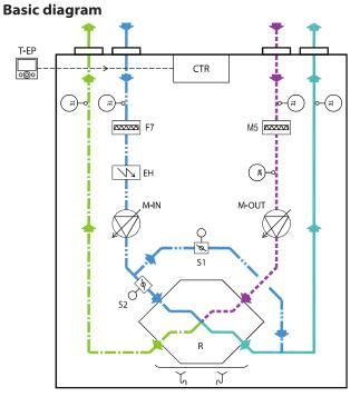
M-IN = Supply fanM-OUT = Extract fan S1 = Main by-pass damper motor S2 = Secondary by-pass damper motor R = Heat recovery system = fresh air = supply air = extract air = exhaust air = micro pleat filter = remote or on board control = electric pre-heater optional only required for cold climates = temperature sensor = humidity sensor central demand control = condensate drainage
