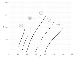
X = Nominal flow rate A = Available static pressure [Pa] B = Power absorbed [W]
