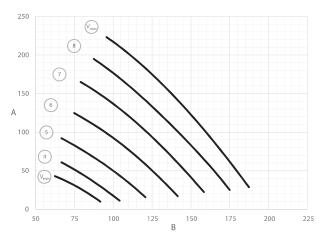
(X) = Control voltage A = Available static pressure [Pa] B = Air flow [m<sup>3</sup>/h]
