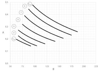
$\bigotimes$  = Control voltage A = SFP [W/m<sup>3</sup>/h] B = Air flow [m<sup>3</sup>/h]
