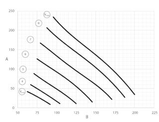
$\bigotimes$  = Control voltage A = Available static pressure [Pa] B = Air flow [m<sup>3</sup>/h]
