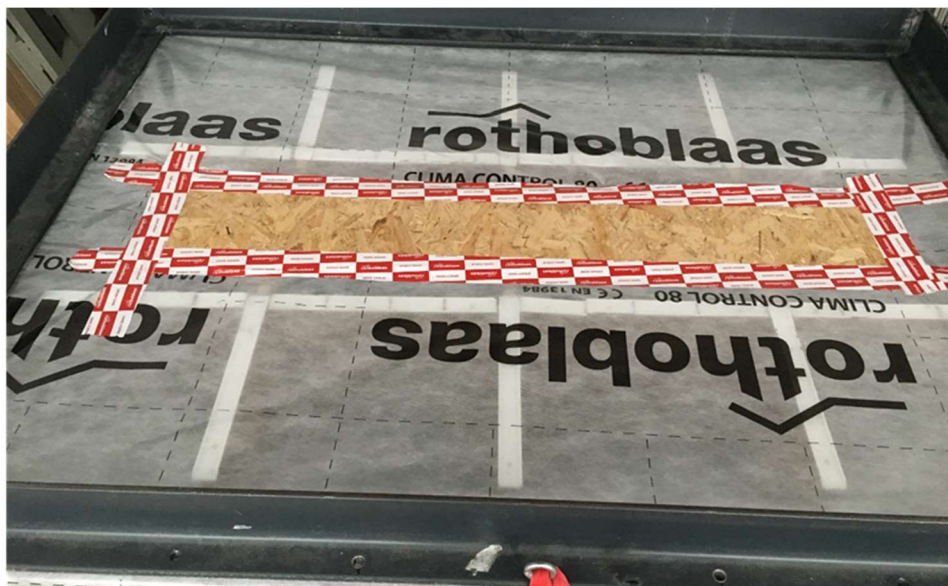
Fig. 3: OSB panel joined to the membrane on all four sides using Speedy Band.
