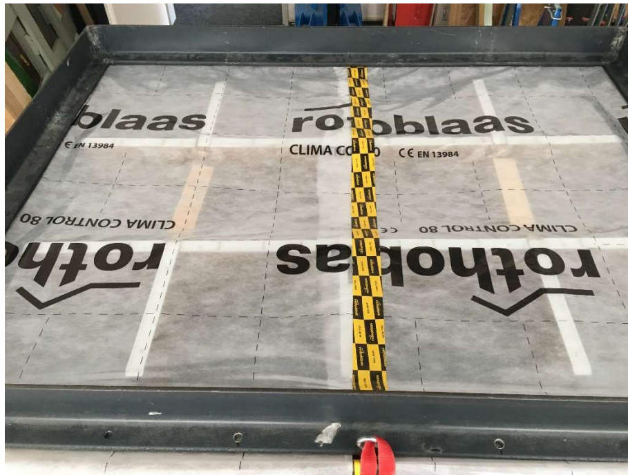
Fig. 1: Connection of two pieces of membrane with Seal Band adhesive tape.
