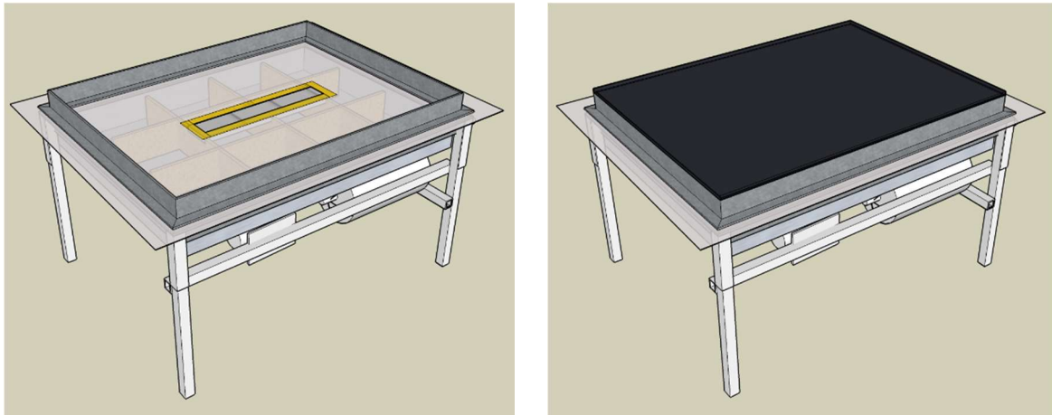
Fig. 5: Sketch of the test apparatus with the clamped membrane and inserted panel which is joined to the membrane with adhesive tape (yellow) (left). Test apparatus sealed with the cover panel for determining the test stand leakage (right).
