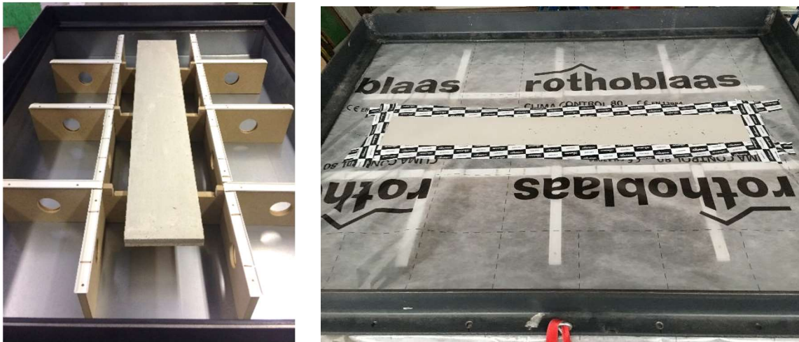
Fig. 2: Fixture for panels in the test apparatus with the concrete slab in position (left). The fixture for the panels simultaneously serves to support the membrane at negative pressure. Adhesion of the concrete with the membrane using Flexi Band(right).
