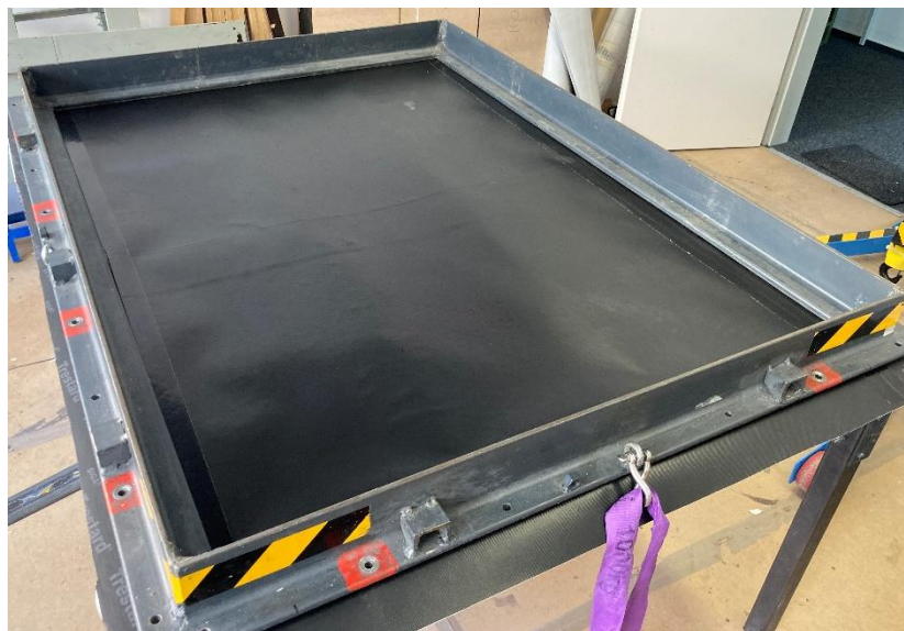
Fig. 5: Test apparatus with clamped membrane (membrane to membrane joint by overlap)
