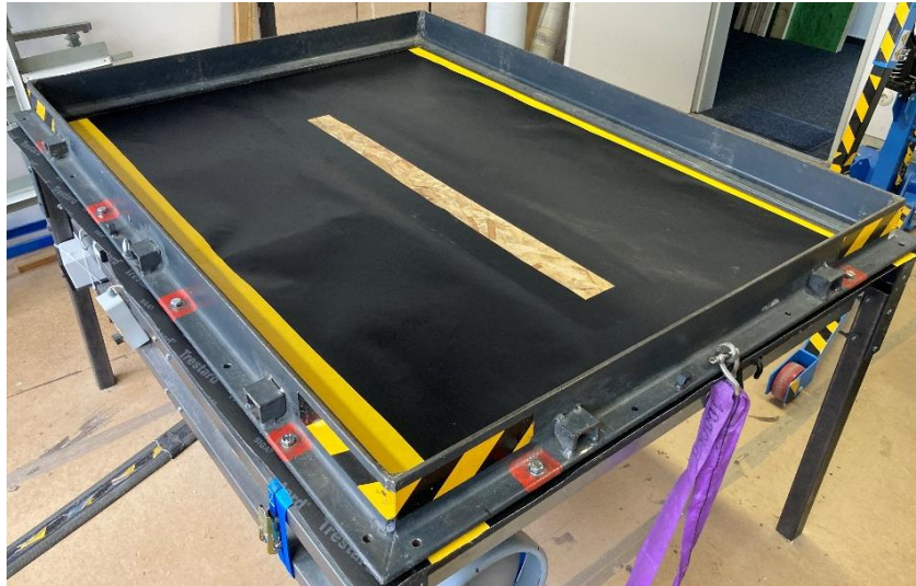
Fig. 2: OSB panel joined to the membrane on all four sides by overlap.
