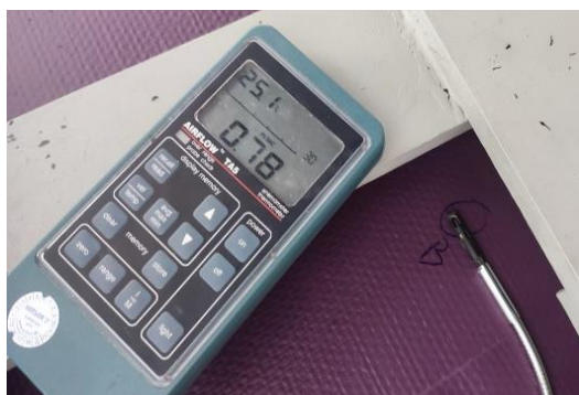
Fig 17: Air leakage is visualised with the help of an anemometer.
