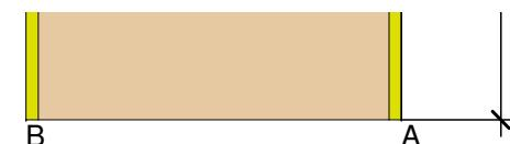
$$\psi_{A-E,C,*} = \frac{\Phi}{\Delta T} - U_1 \cdot b_1 - \frac{\Phi_2}{\Delta T} = \frac{14,931}{30,000} - 0,192 \cdot 1,010 - \frac{8,341}{30,000} = 0,025 \text{ W}/(\text{m} \cdot \text{K}) \psi_{A-E,C,*} = \frac{\Phi}{\Delta T} - \frac{\Phi_1}{\Delta T} - U_2 \cdot b_2 = \frac{14,711}{30,000} - \frac{8,341}{30,000} - 0,192 \cdot 1,010 = 0,018 \text{ W}/(\text{m} \cdot \text{K})$$
