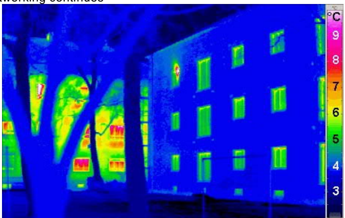
The dark colours on this thermogram of a Passive House, at right, shows how little heat is escaping compared to a traditional building to the left (wikipedia).
