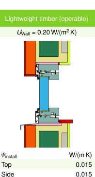
Bottom 0.021  $U_{W \text{ installed}} = 1.04 \text{ W}/(\text{m}^2 \text{ K})$
