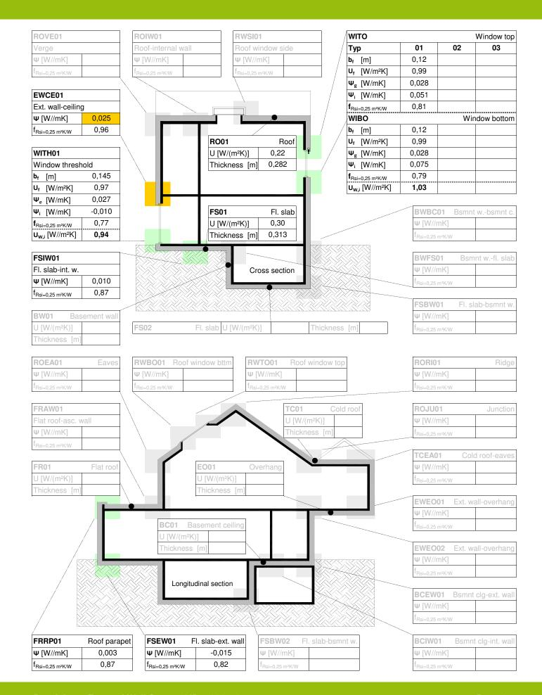
Page 2/4 Passivhaus External Wall System | ID: 1236cs04
