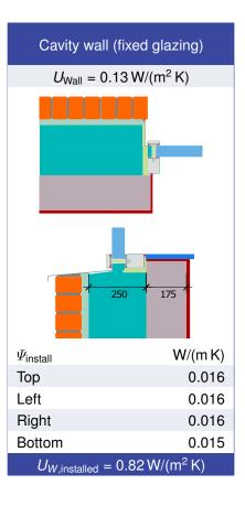
$<sup>^{1}</sup>$ Includes $\Delta U = 0.23 \text{ W/(m}^{2} \text{ K)}$ . Determined through 3D FEM simulation
