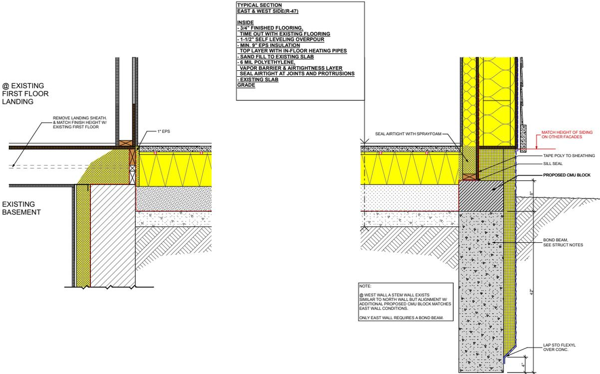
Typical North addition stemwall and basement connection
