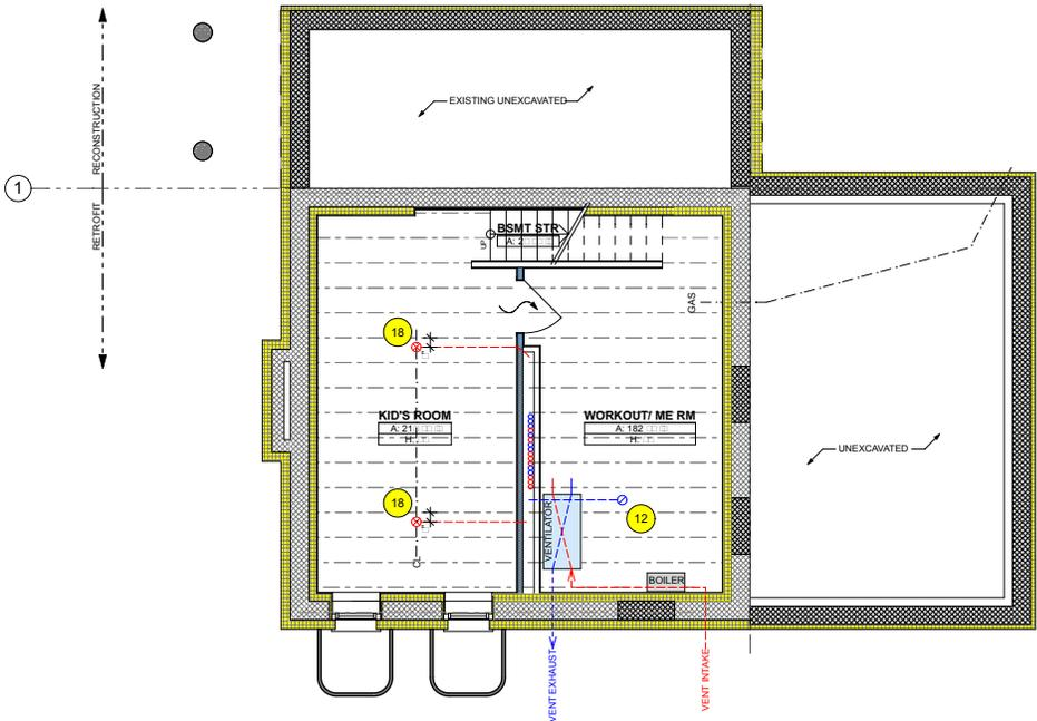
Basement level ventilation plan
