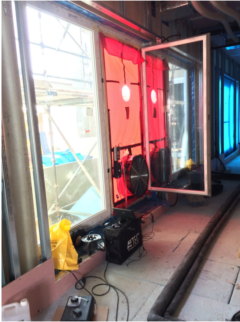
preliminary pressure test before completion (EIFS, counterwalls, screeds were missing)
