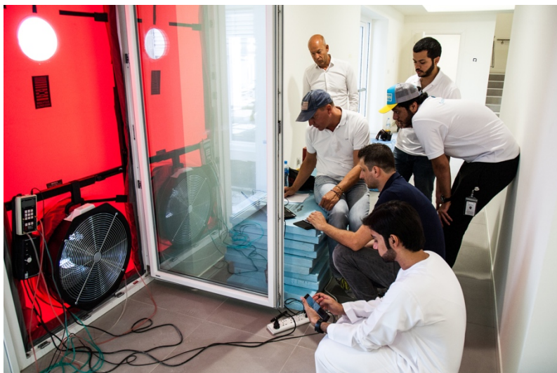
final pressure test at the presence of client (MBRSC) technicians
