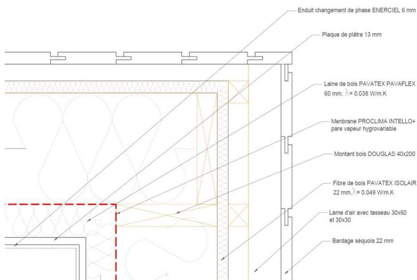
The walls are in continuation with the existing private house. So the structure is similar as for the wall framework, that's why this is the less isolated face. This wood complex is composed of external woodfiber of 22 mm, then 200 mm of cellulose wadding, and to complete, 60 mm of flexible woodfiber.
