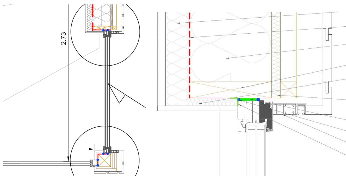
The windows are positioning closer to the exterior, to receive maximum sun light and heat, but also to be more performant as possible. I did a THERM calculation to
