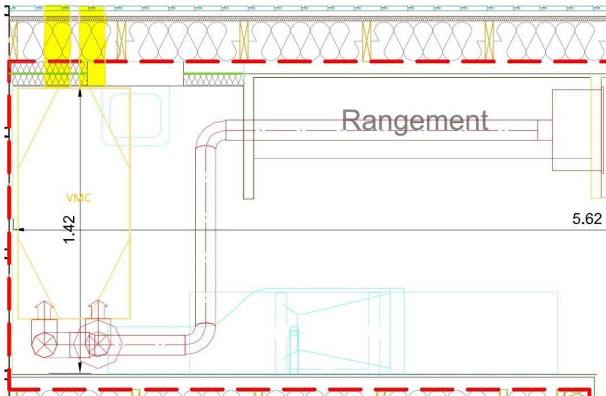
For the secondary ducts inside the project, I used a LINDAB ducts spiral tubes. Those strong and jointed tubes are only 5 meters. Most of them are hidden near the ventilation, but a small part going to the desk is keeping viewed
