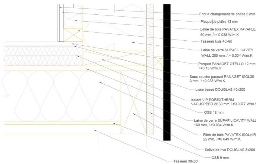
In the research of Japanese architecture, I choose for foundations some stones piles, the wood joist are fixed on it. It is also more easy to use natural insulation, between the joist with cellulose wadding of 160 mm. To complete insulation, I used VIP (vacuum insulation Panel) because the ceiling height was already low. Those panels are really high insulation, with a lambda of 0.0077 W/m.K.
