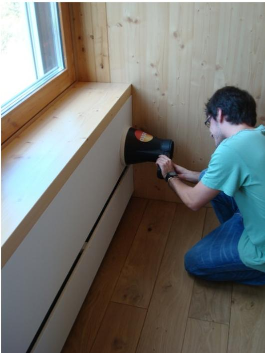
Reading the air flow rate in a supply air valve
