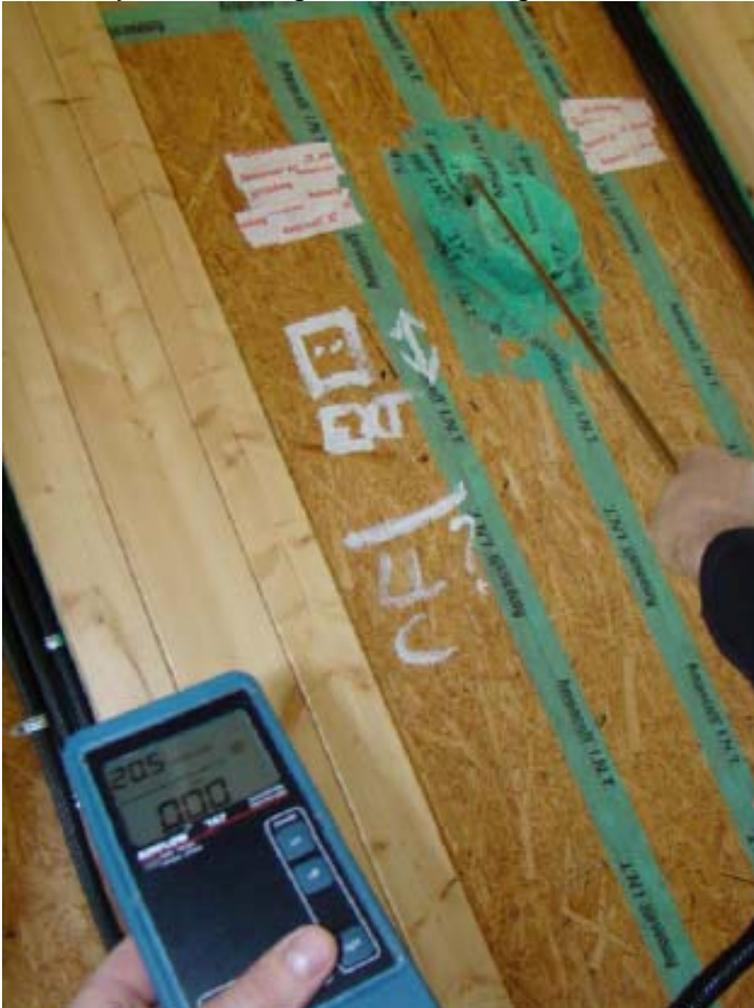
*Control of infiltrations during the first Blower-Door test*
