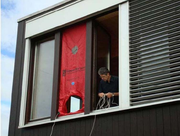
The Blower-Door test was done in November 2012, giving a result of  $n_{50} = 0.61/h$ . With the objective of measuring infiltrations through the ground floor entrance door, the Blower-Door machine was positioned in one of the windows of the living room, on the first floor.
