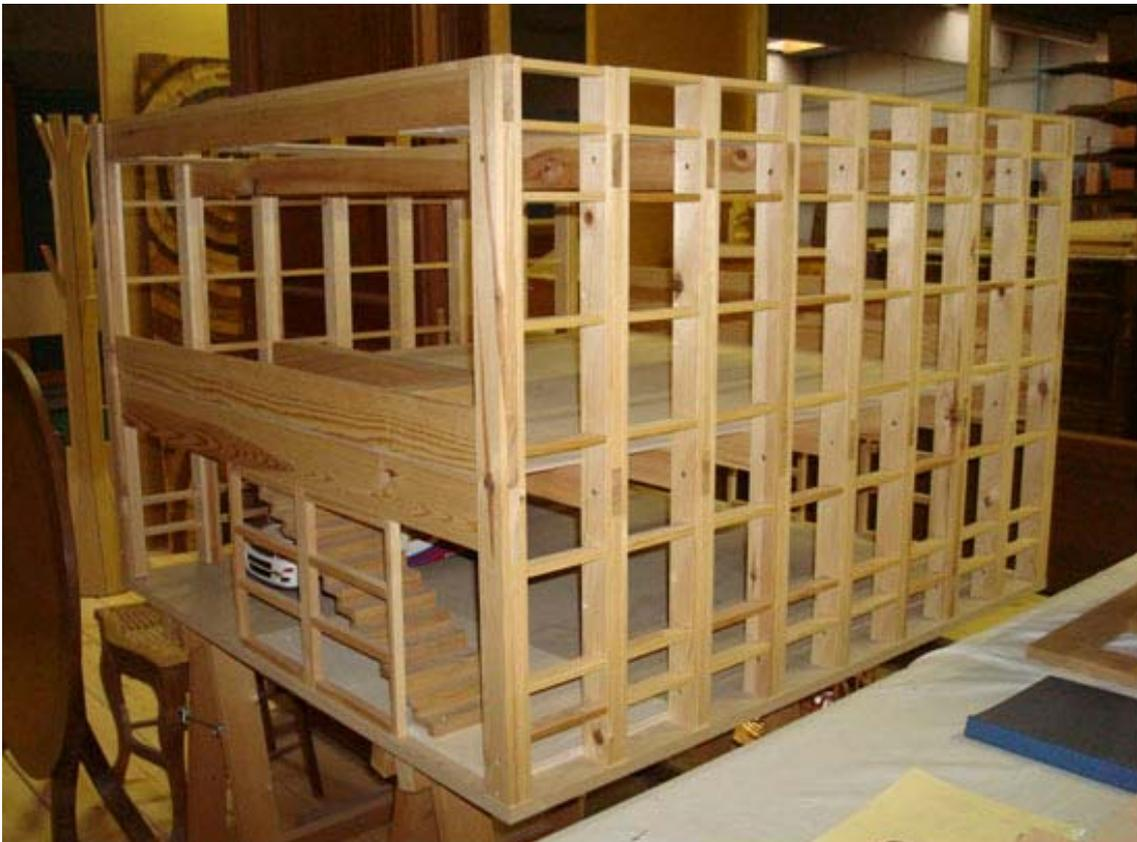
*Structural model of the building, scale 1/10*
