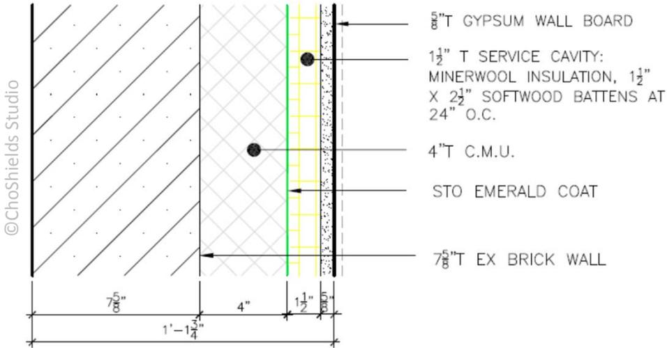
On the existing brick party walls, we added an additional wythe of 4" CMU block as part of the structural remediation. Although these walls were adjacent to another building, we insulated all 1 1/2" service cavities 3' in from exterior exposed walls.
