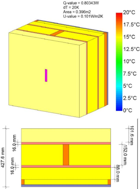
This wall assembly is the same as assembly no 1, the timber frame wall, except that since the juncture between the existing masonry and the new vertical extension occurred approximately 4' above the finish floor, there was room to add extra insulation on the interior of the upper part of the wall. We submitted the thermal performance of this assembly in PSI Therm as part of our certification.
