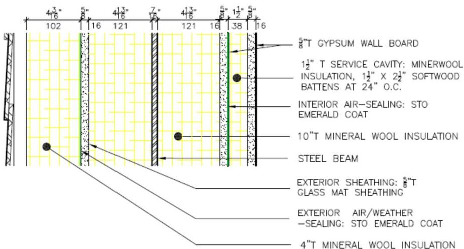
All cavities in the rear addition steel moment frame were filled with mineral wool insulation. The wall was insulated on the interior with a  $1\frac{1}{2}$ " service cavity and on the exterior with 4" continuous mineral wool.
