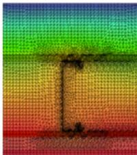
The 1-hour fire-rated roof assembly has an average of 7" deep continuous polyiso insulation under the modified bitumen roof membrane. The structural roof deck is made from light gauge steel joists at 16" o.c. with mineral wool cavity insulation.
