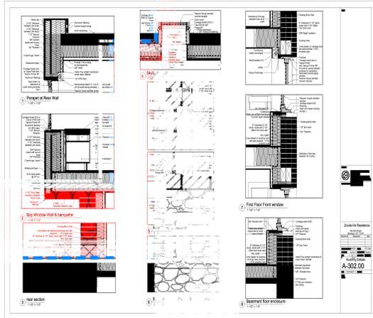
The ground floor is built over an uninsulated basement. Two inches of foil-faced EPS foam were installed under the existing floor joists. Joist bays were filled with dense packed cellulose insulation.
