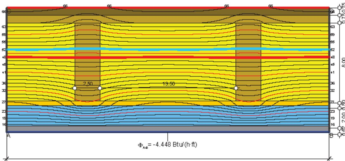
$$U_{\text{eq}, A-B} = \frac{4.277}{30.000 \cdot 0.813} = 0.175 \text{ W/(m}^2 \cdot \text{K)} = 0.0309 \text{ Btu/(h}\cdot\text{ft}^2 \cdot \text{F)}$$
