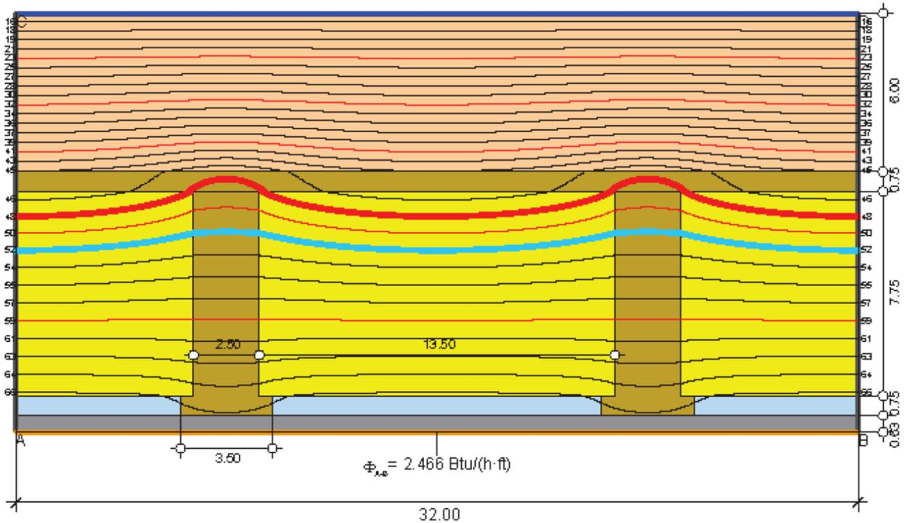
$$U_{\text{eq},A-e} = \frac{2.371}{30.000 \cdot 0.813} = 0.0972 \text{ W}/(\text{m}^2 \cdot \text{K}) = 0.0171 \text{ Btu}/(\text{h}\cdot\text{ft}^2 \cdot \text{F})$$
