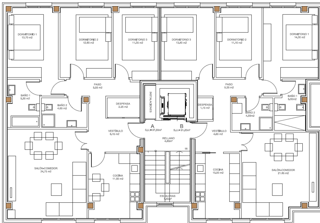
Third floor Source: Construcciones Zorzano
