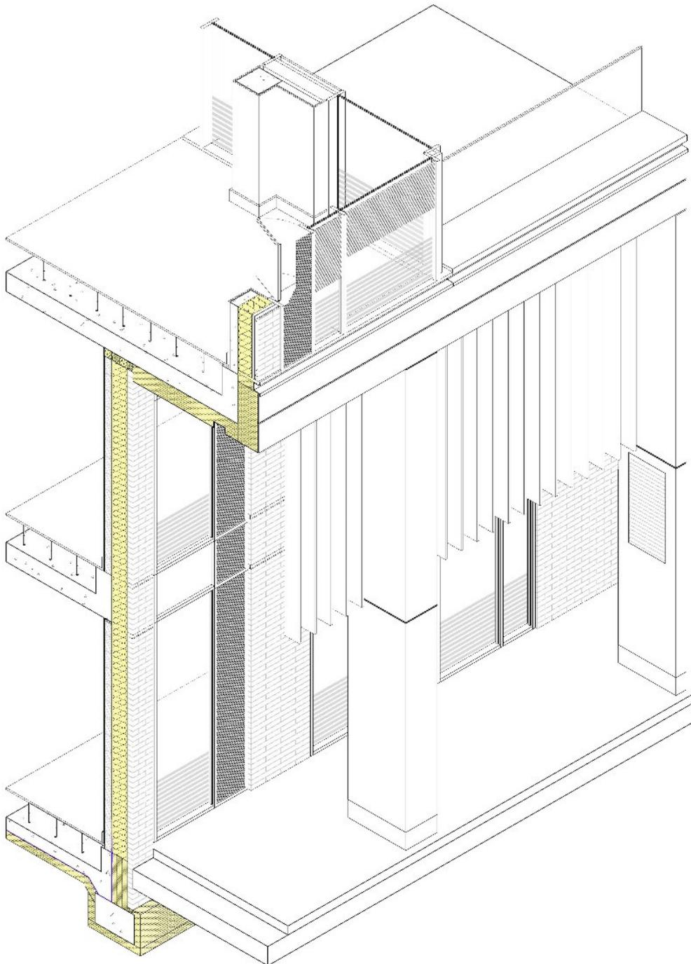
Drawing showing ground floor/wall connection and upper floor/wall connection
