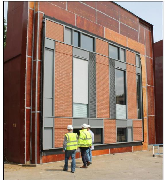
Envelope Mock-up, Testing and Inspection for Air-tightness and Water at Wind-Techs Facility
