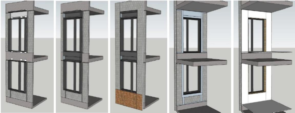
103mm Ibstock Red brickwork externally, followed inside by 300mm cavity with Knauf Earthwool Dritherm 32 Ultimate mineral wool insulation, 140mm medium density blockwork, 13mm wet plaster internally. TeploTies to cavity masonry. Foamglass loadbearing insulation to base of masonry.
