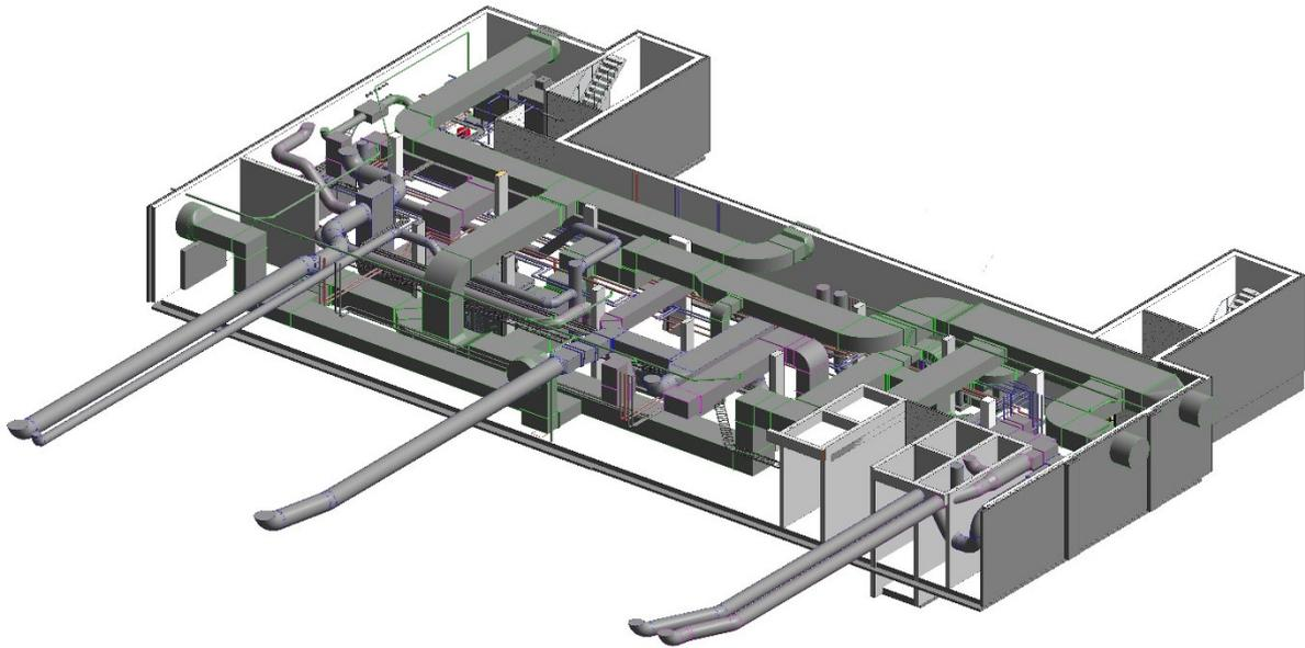
Schematic of basement AHU layout
