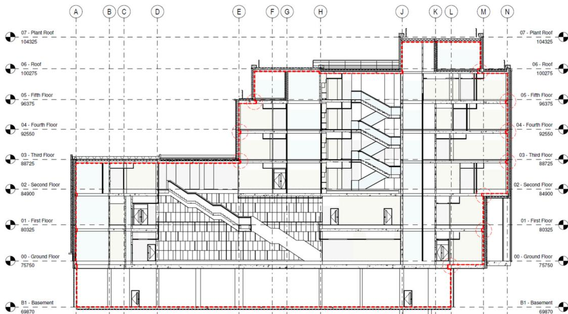
Cross-section showing continuous air-tightness line at early stage
