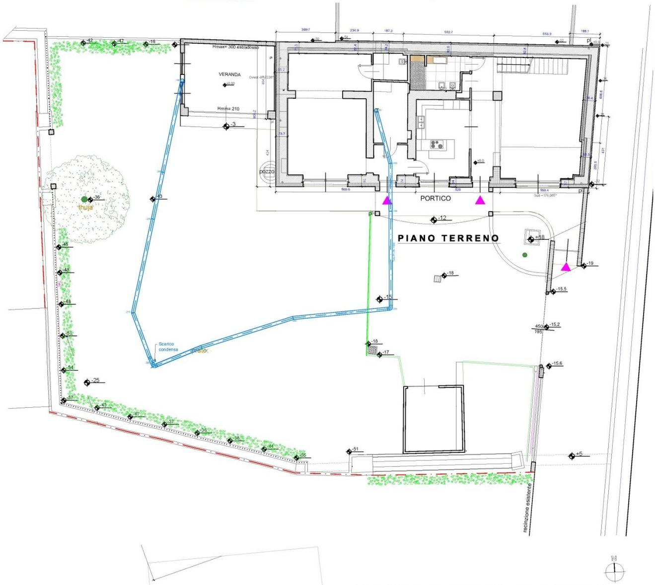
air-ground exchanger diagram
