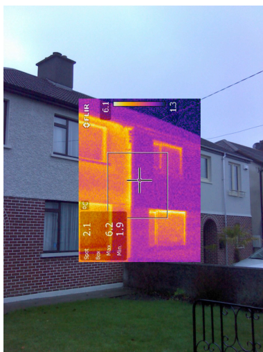
Fig 24 thermal image overlay of photo elevation showing temperature differences
