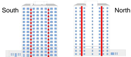
The technical balconies are located at each level on the North and South façades of the buildings and are used to support the external conditioning units.
