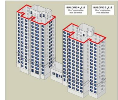
**Fire locks** – for fire safety reasons, there is a fire lock made of mineral wool at the perimeter of the roofs.
