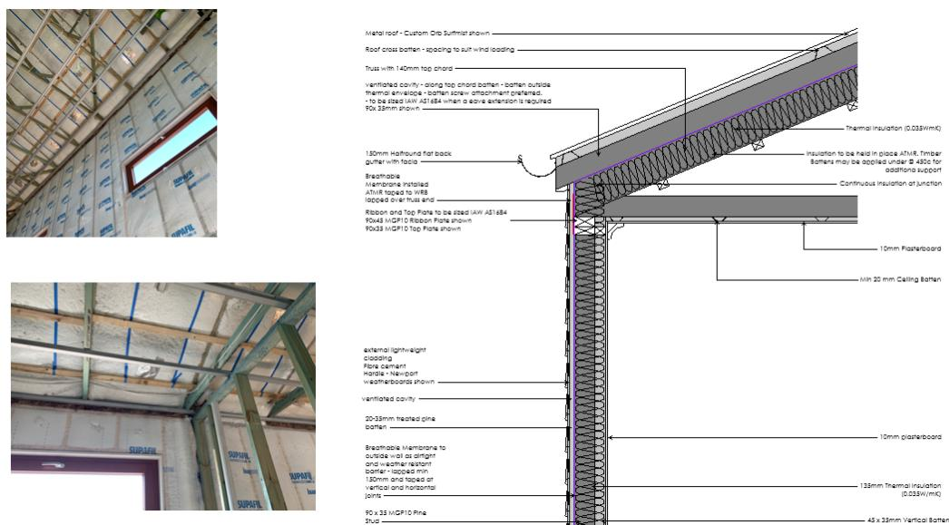
Figure 4 - Roof Wall Junction
