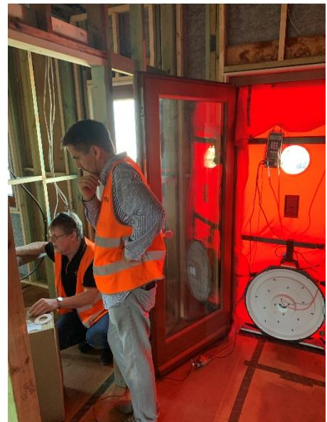
Figure 2 - Airtightness Testing Final Result (left) Image of the initial blower door test (right)
