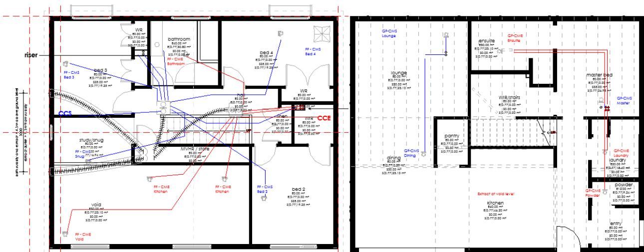
Figure 6 - MVHR Plan - Firstfloor and ceiling (left) Ground floor ceiling (right)
