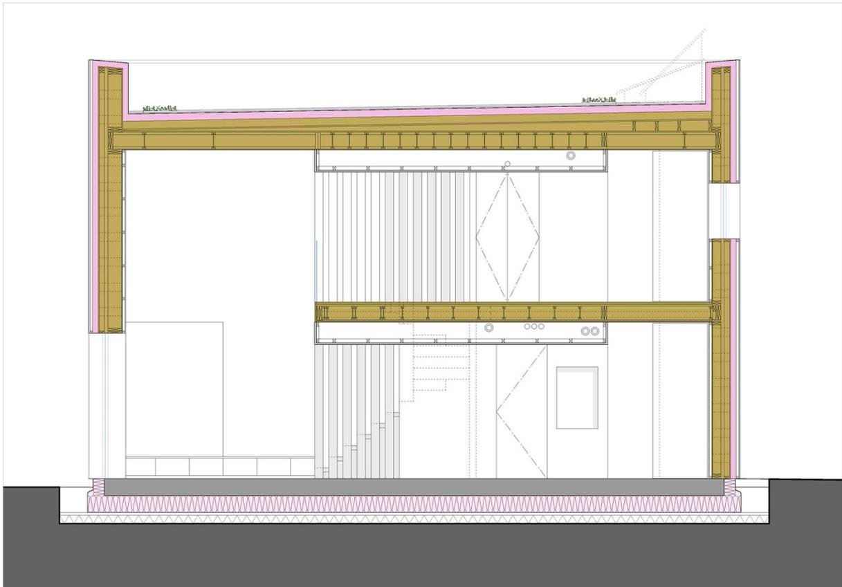
The cross section clearly shows the insulated raft foundation by Isoquick, the twin-wall timber frame construction (shown in brown) and the external wrap of continuous Gutex insulation (pink), which also extends up and over the parapet to ensure complete continuity.
