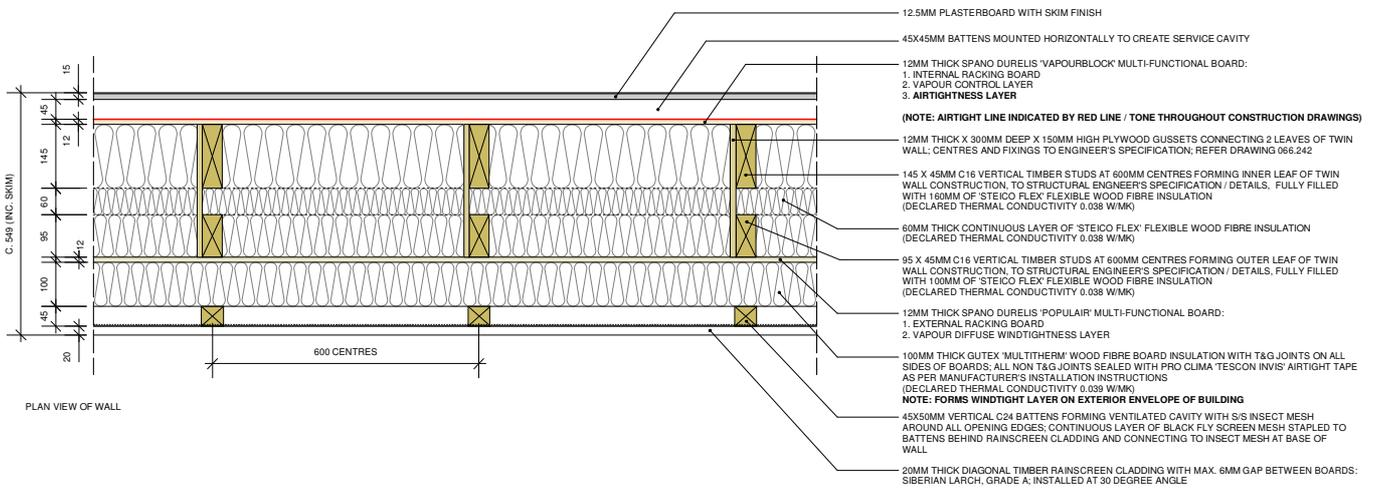
EXTERNAL WALL TYPE 2: TWIN-FRAME 245MM INNER STUD
