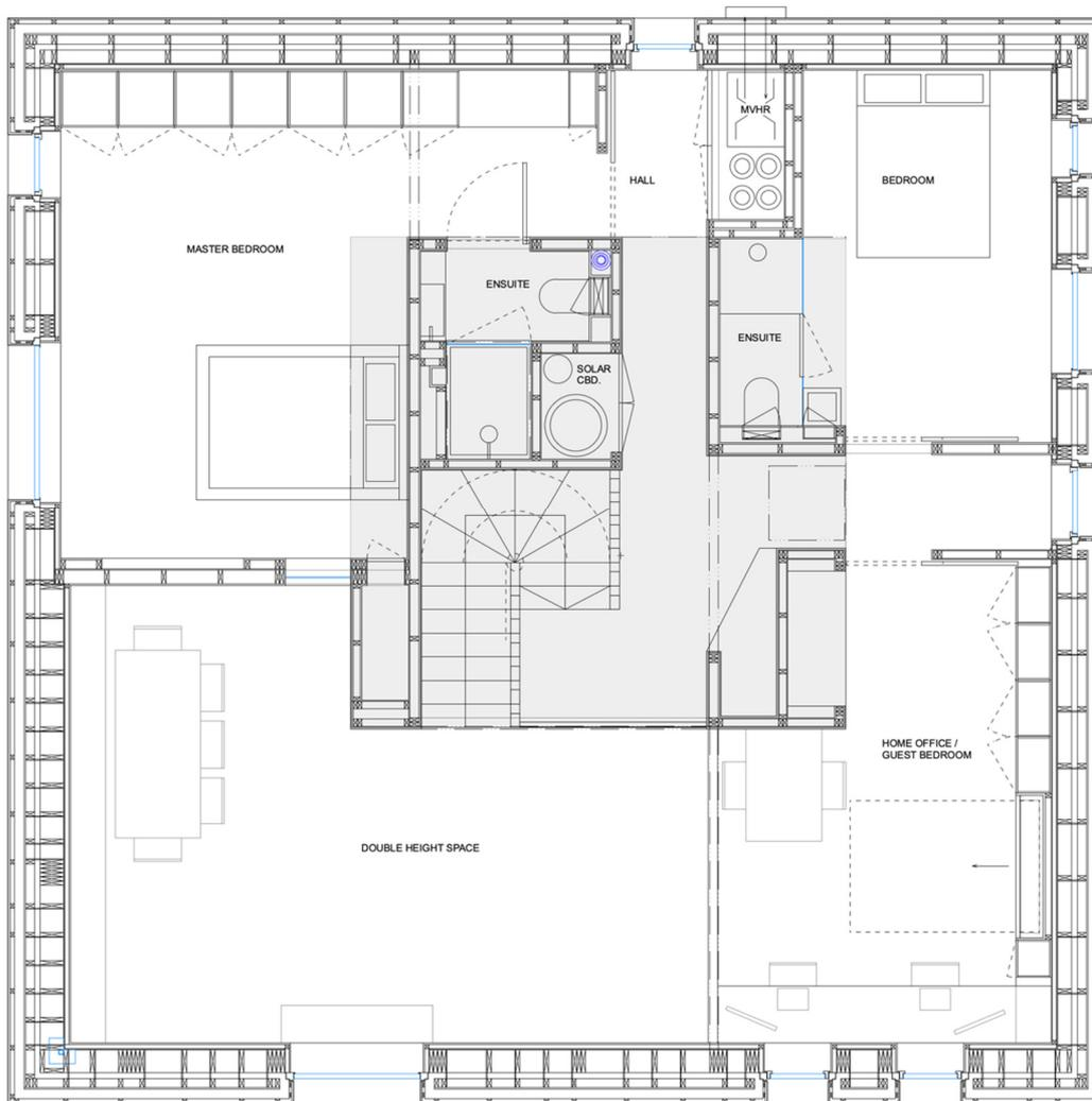
The First Floor Plan: again there are minimal windows to the north. Two more bedrooms are orientated either due west or east facing, both with ensuites contained within the central service core.
