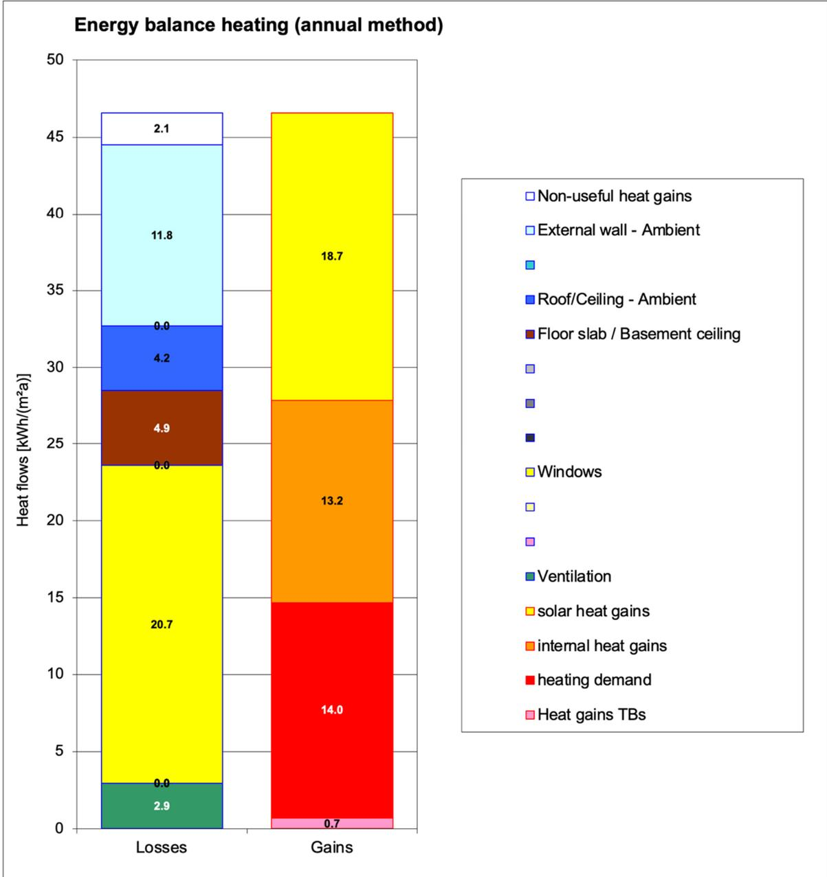
The energy balance (annual method) shows that the losses from windows (20.7kWh/m<sup>2</sup>.a) are under half of the total losses, and these are almost balanced by the solar gains (18.7kWh/m<sup>2</sup>.a).
