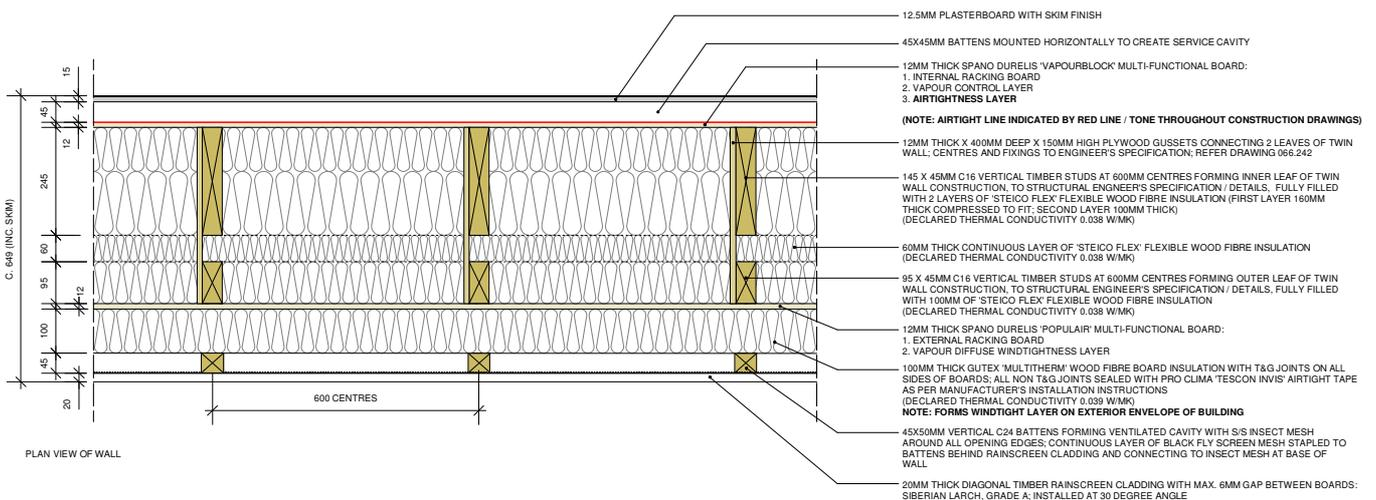
This drawing shows the external wall construction in both the areas with 145mm load-bearing studs, and 245mm load bearing studs (double height). The whole wall construction is filled with wood fibre insulation batts.
