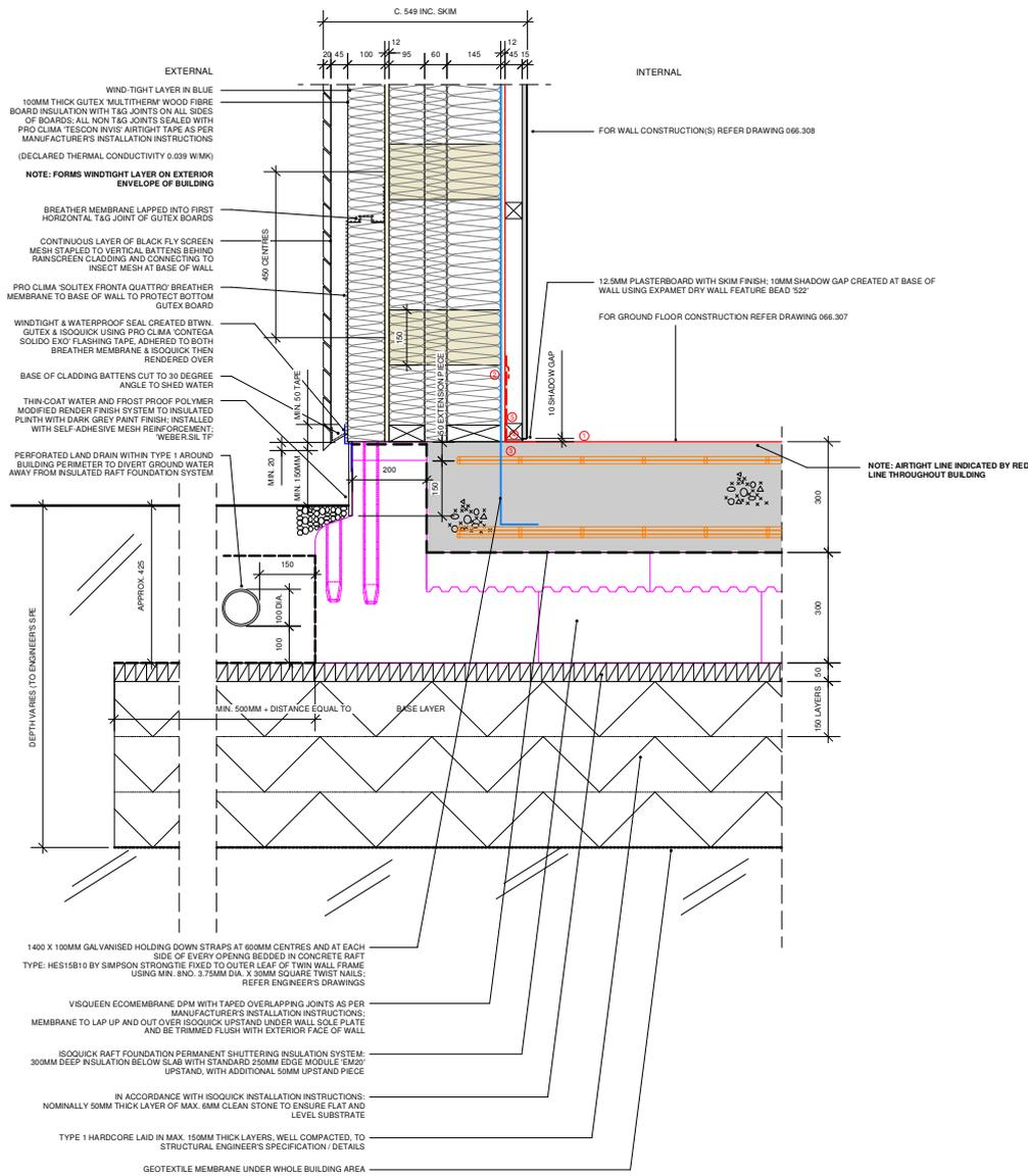
TYPICAL SECTION THROUGH WALL / GROUND FLOOR JUNCTION WITH WALL TYPE 1: 145MM & 95MM TWIN WALL TIMBER FRAME (NOTE: FOR WALL TYPE 2 DETAIL, REMAINS CONSISTENT)
