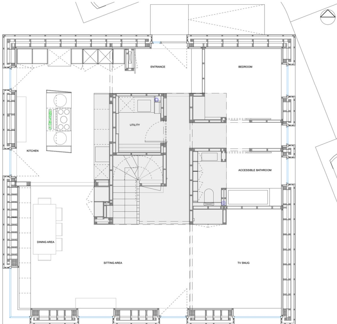
The Ground Floor Plan: to the north is the entrance door with a single narrow window adjacent. In the north east corner is a double bedroom, and immediately below that is the accessible bathroom. In the south east corner is the TV sitting space, and in the south west corner under the double height are the dining and secondary sitting spaces. In the north west corner is the kitchen. The whole of the ground floor, with the exception of the bedroom and bathroom, is open-plan.
