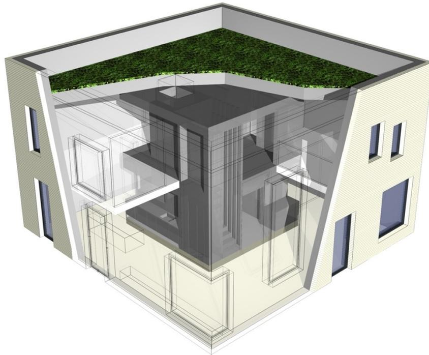
This 3-D cutaway, looking from the south west corner, also shows the inner service core, the parapet and sedum roof covering.
