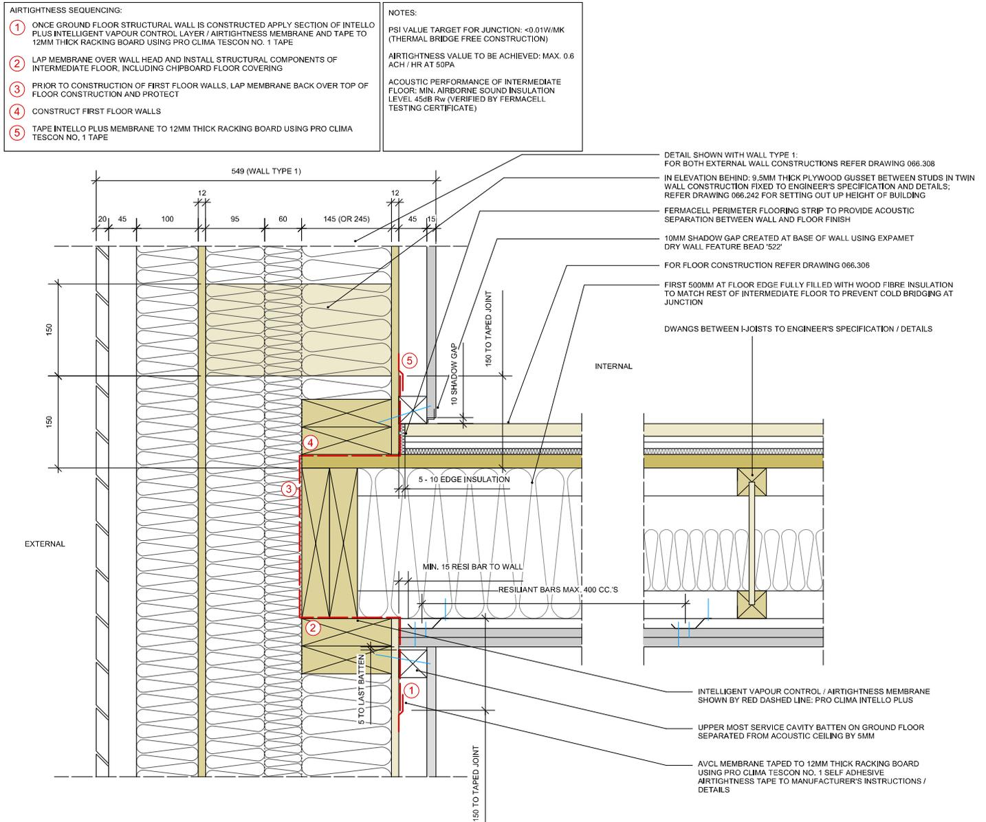
TYPICAL SECTION THROUGH INTERMEDIATE FLOOR JUNCTION WITH WALL TYPE 1
