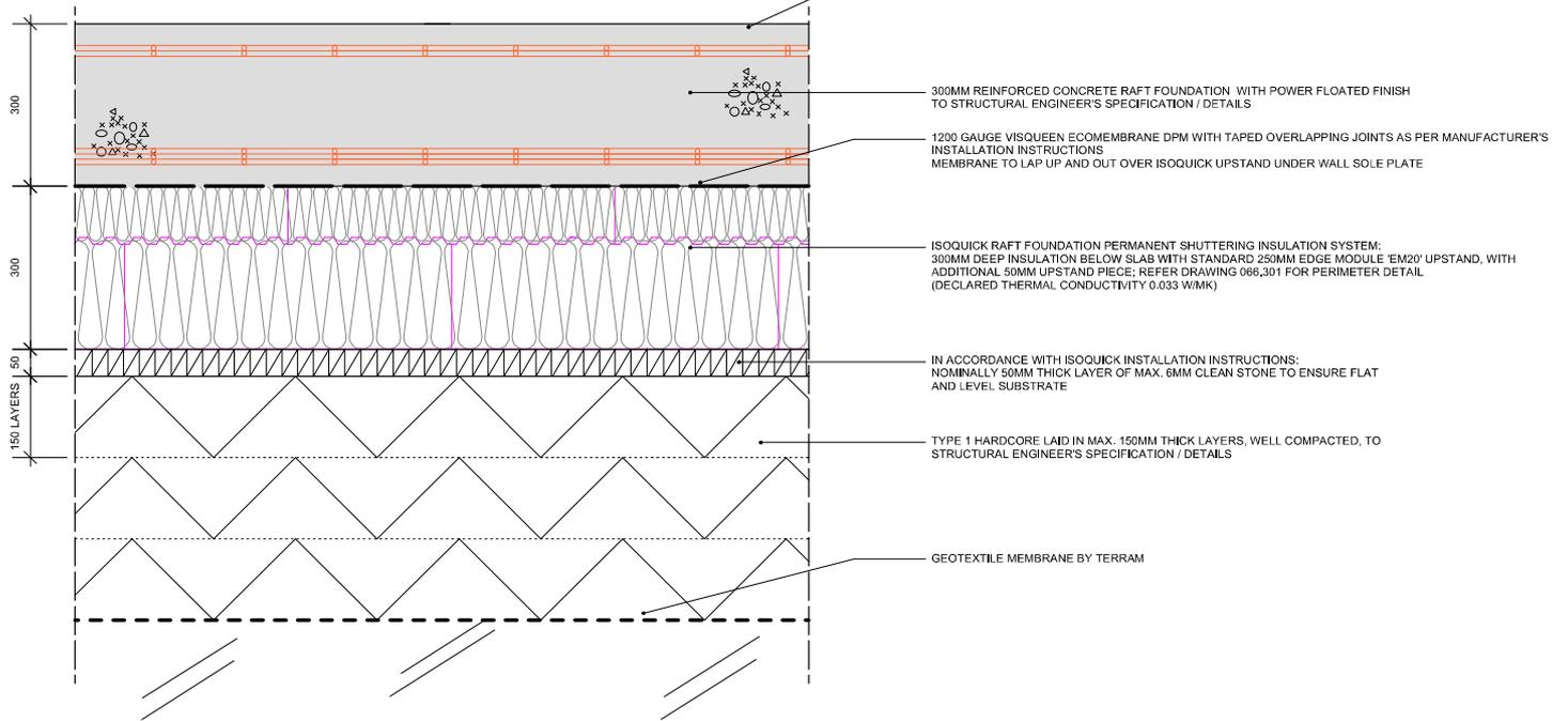
These 2 drawings show the construction of the ground floor slab insulated raft formwork where it meets the external wall (top) and the floor construction itself (above).
