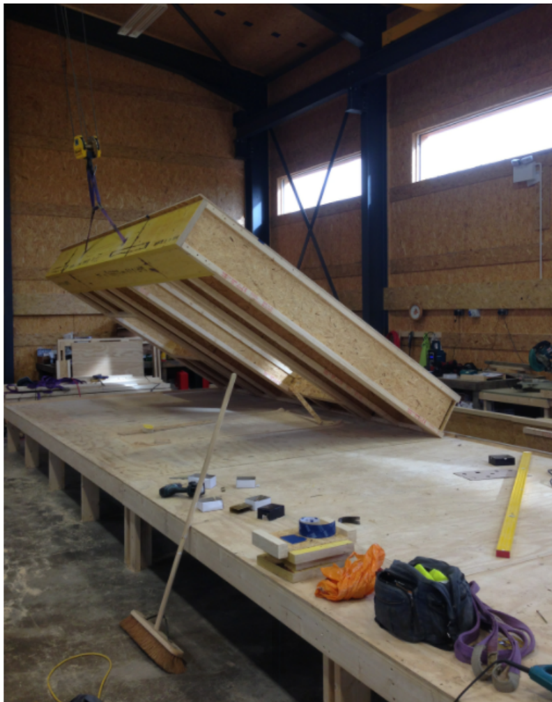
Figure 17 – Timber wall panels being constructed in the factory
