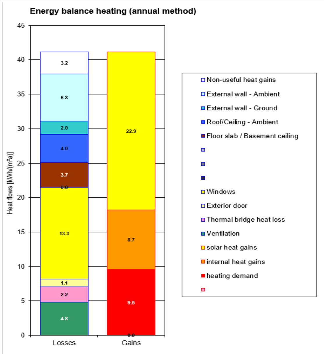
Picture 26: The heating demand balance of the single-family house, calculated by the PHPP.
