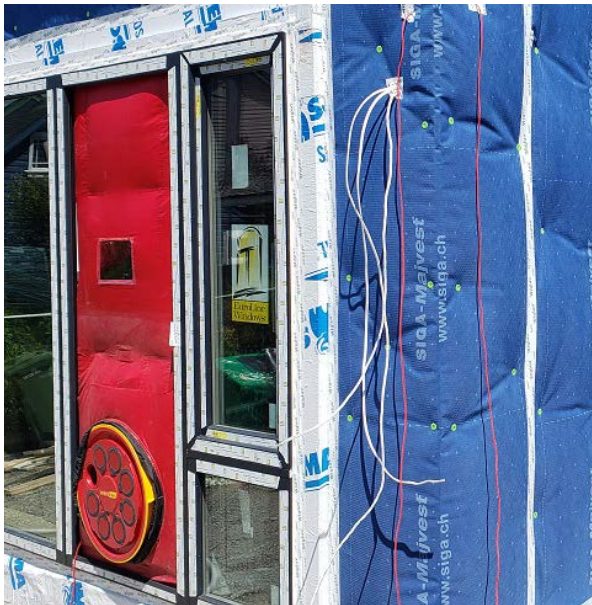
Initial Blower Door Test 05-28-2020 Siga Majvest taped to window frames & SAM
