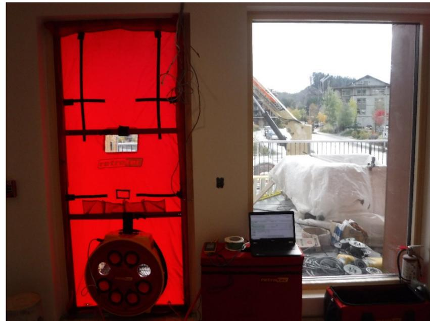
TEST FAN SETUP AT THE MAIN ENTRANCE ON THE GROUND FLOOR.
